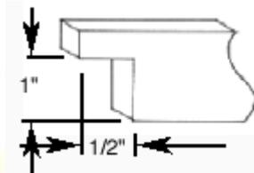
Once cut to shape, sand the piece to round off the edges and then glue it on top of the two plywood sides, half way between the front and back.
