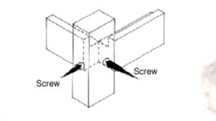
Ideally, the side supports should be attached at even intervals (every 30"), but you can modify this to suit your own requirements. Repeat for the other side, taking care to ensure that the routed groove points towards the middle of the shelving unit. Take the time to ensure that all joints are square; otherwise you may end up with a shelving unit that leans!
