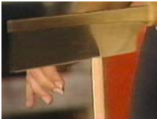
Cut a slot in the end of the dowell using a back saw.
