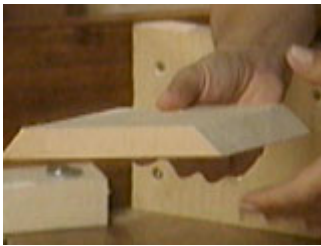
Cut four corner braces with mitred ends
