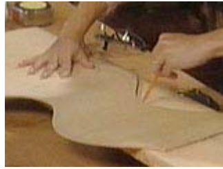
Make a curvy design from cardboard and transfer it to the undercarriage
