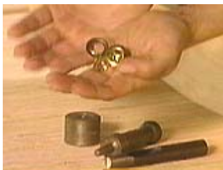
Grommets, block or seat, set and punch - top to bottom.
