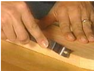
Use a cornering tool, sand paper or a plane to remove the sharp edge.
