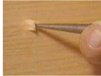
Drive a finish nail into the spot and set it a bit deeper than the wood surface using a nail set
