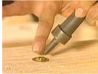
Place the grommet on the block or seat and then use the set to crimp.
