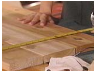
Measure the width of the bottom boards and cut a side board to fit.
