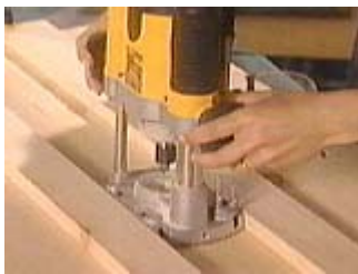
Set up a guide fence on either side of the router for the 'V' groove
