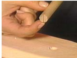
Cut the slot deep enough to make it easy to slip in the hole.
