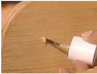
Glue the shaving back in place with high-tack fish glue
