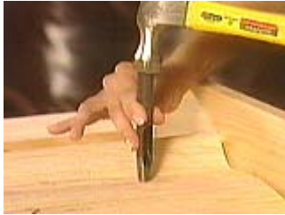
Use the punch to cut a hole for the grommet.
