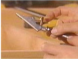
For blind nailing, use a tiny plane
