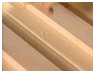
Test for depth and rout a groove along each joint on the back
