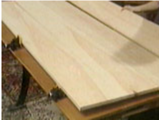
Place the four boards in pipe clamps
