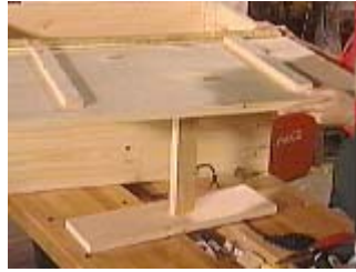
Use the jig to help hold up the lid while attaching the hinge.
