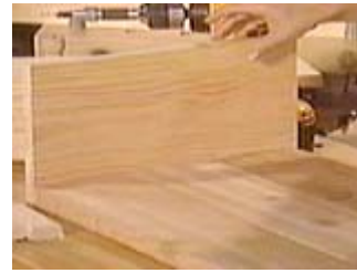
Cut the length of the side boards to match the width of the three bottom ones.
