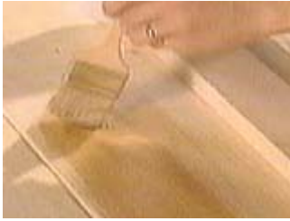
Apply a water based aniline stain with a brush
