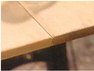
For less color on end grain (left) spray with water first
