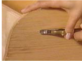
Lift a shave of wood in the place where the nail goes
