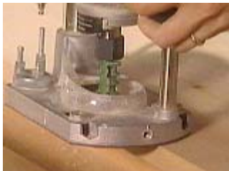
Plunge router with beading bit
