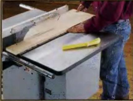
**1** Start rip cuts with your left foot against the front left corner of the saw base. Feed the workpiece with your right hand, and use your left hand to keep the workpiece snug against the rip fence. Use a pushstick whenever a workpiece requires your hand to be closer than 6 in. to the blade.
