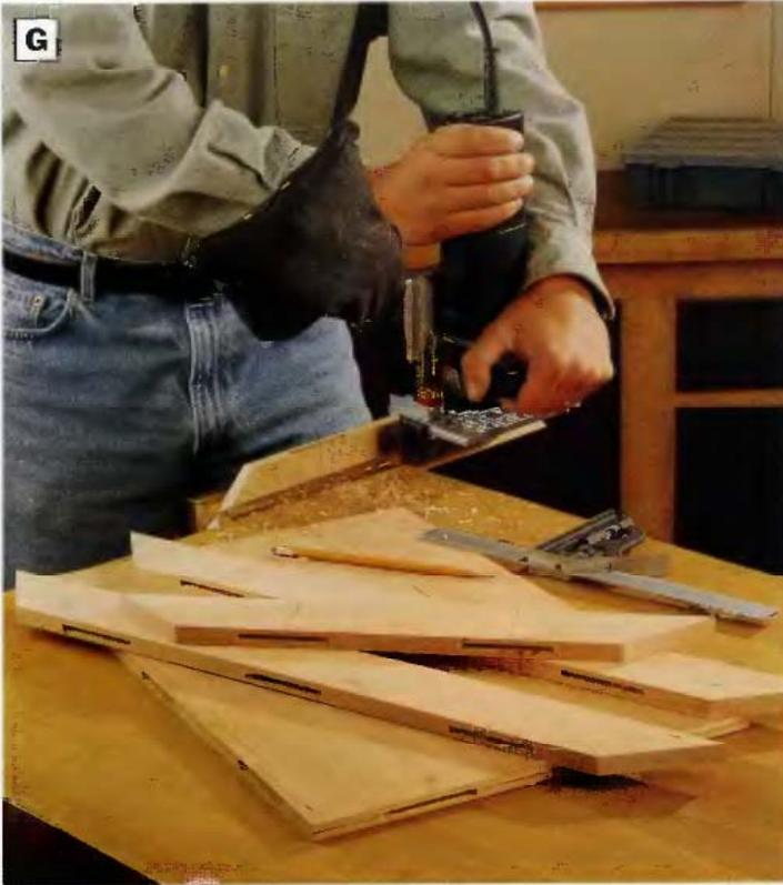
**PHOTO G:** Lay out and cut #20 biscuit slots to join the frame side and end pieces to the bottom panel. Clamp the parts in a bench vise to hold them securely when you cut the slots.
