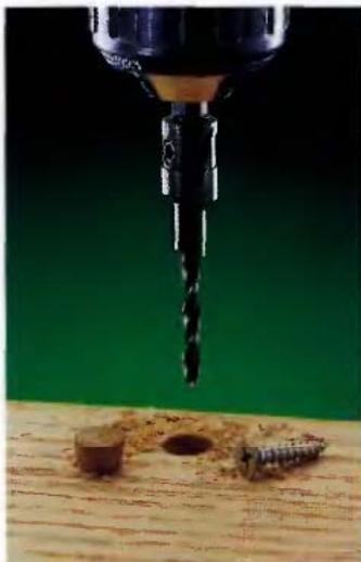
A COUNTERBORE BIT can drill a pilot hole, shank hole and counterbore hole all at the same time.
