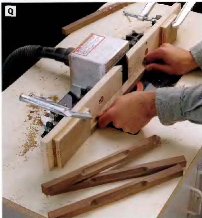
**PHOTO Q:** With the bit spinning, feed the workpiece up against the fence, making sure it contacts the start block. Then, feed it toward the stopblock until the cut is finished.
