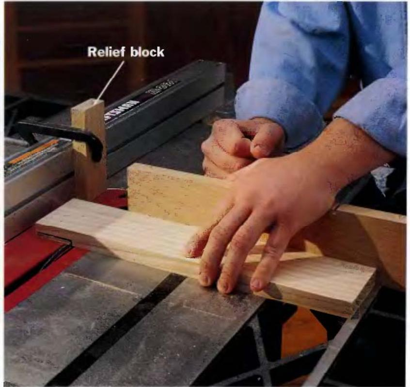
**2** Cut the shoulders of the tongues on a table saw, using the miter gauge to feed each workpiece past the blade. Clamp a relief block to the fence and measure out from its position to the blade to set up the cut.
