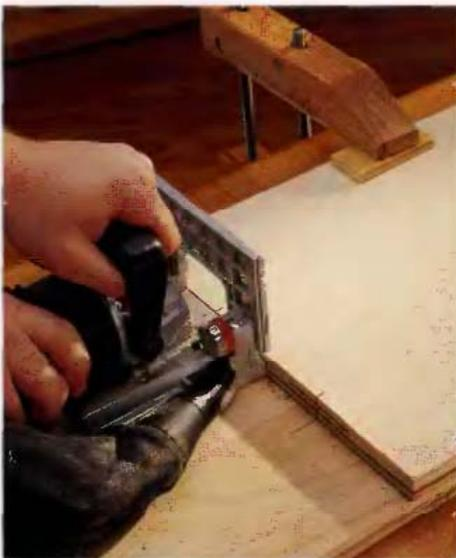
**1** Lay out the position of the two mating parts using a square (note whether you're marking the top or bottom of the workpiece). Set the mating workpiece in position against the mark. Draw a perpendicular reference line on both workpieces at each biscuit location. With the workpieces clamped together and secured to your worksurface, align biscuit joiner with the reference lines and cut the slots in one workpiece.
