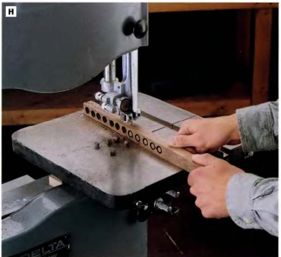
**PHOTO H:** Cut 16 to 20 plugs with the plug cutter, then resaw the walnut stock to about  $\frac{3}{8}$ -in. thick to release the plugs.
