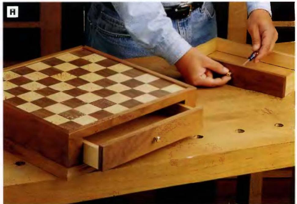
**PHOTO H:** After applying three coats of satin polyurethane, install the knobs on each drawer. Although we don't show it here, you may also want to add catches or turnbuckles for holding the drawers closed for transport.
