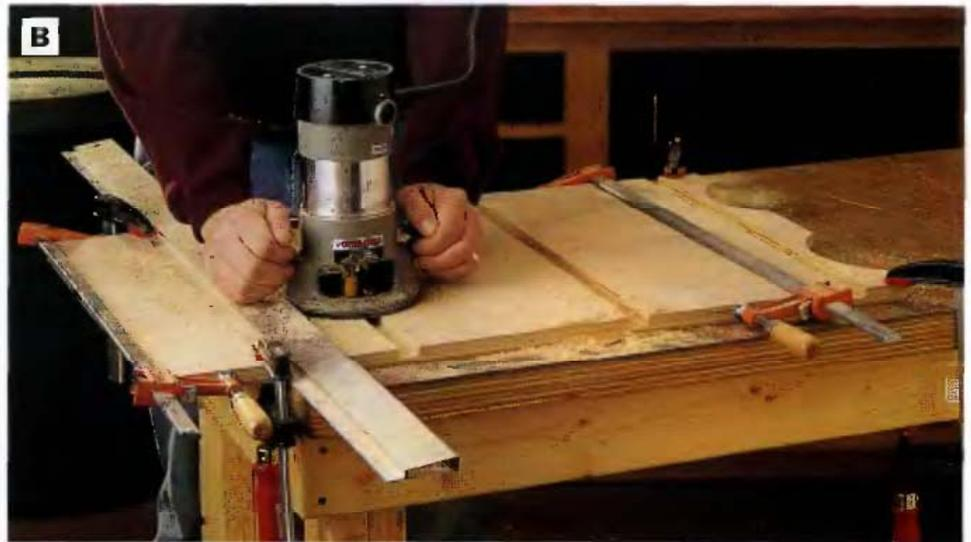
**PHOTO B:** Clamp the sides together side by side, lay out the shelf dado locations and gang-rout the dadoes across both sides. Clamp a straightedge across the side workpieces to guide the router cuts.
