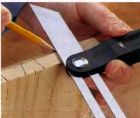
USE A SLIDING T-BEVEL to transfer angles to your workpiece.
