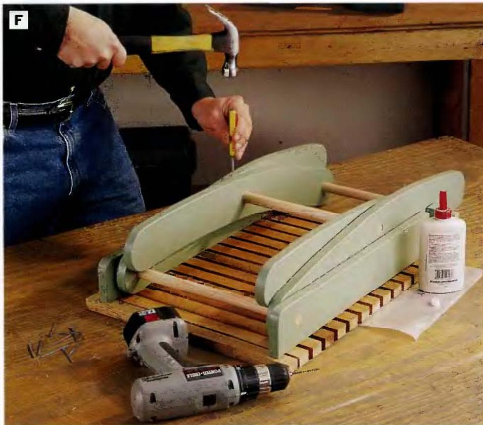
**PHOTO F:** Install the inner legs between the outer legs, and insert the leg pivot dowel through the center dowel holes in the legs. Cut and insert the table lock dowel through the inner legs. Pin the table lock dowel to the inner legs and the leg pivot dowel to the outer legs with finish nails.
