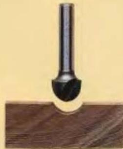
**CORE BOX BIT.** Grooving bit for fluting, veining and carving. Available sizes: 1/4, 3/8, 1/2, 5/8, 3/4 in.; 1/2 in. shank only: 7/8, 15/16, 1 in.
