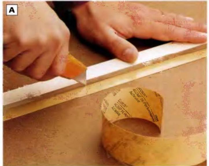
**PHOTO A:** Peel off the protective paper that covers the adhesive backing of the maple veneer and adhere it to the  $\frac{1}{4}$ -in.-thick walnut strips. Trim the veneer to fit the walnut with a sharp utility knife.
