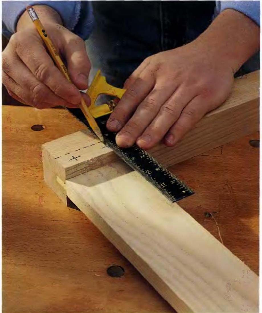
**1** Cut the mortises and tenons, then glue and clamp the joint. Let the glue set up, then lay out the location of the pins with a pencil and combination square. Use at least two evenly spaced pins for each joint, making sure the guide holes are at least  $\frac{3}{8}$  in. from the edges of the boards.
