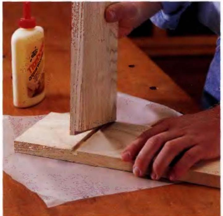
**TEST-FIT THE JOINT** and adjust the thickness of the rabbet ledge by trimming, if needed. Apply glue to both surfaces, then assemble and clamp the joint.
