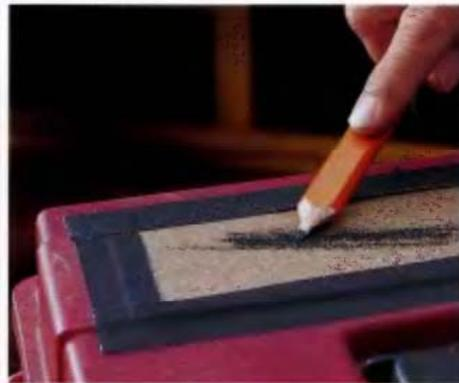
ATTACH MEDIUM-GRIT SANDPAPER to your toolbox to make a convenient and safe sharpener for lumber pencils.
