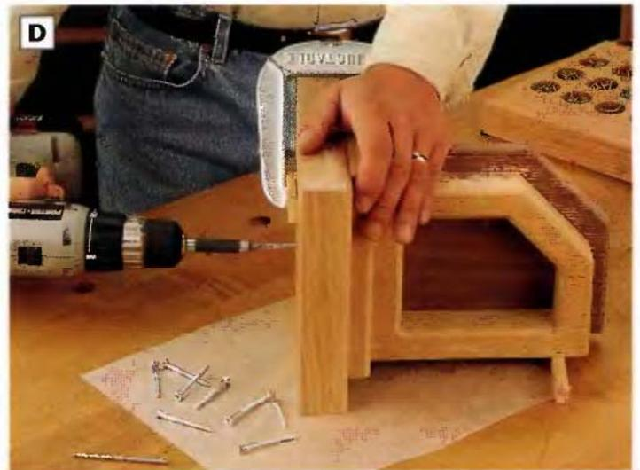
**PHOTO D:** Attach the bases to the frame/base cap subassemblies with glue and countersunk 2-in. wood screws. Clamp and fasten the parts together carefully to keep from spilling the ballast.
