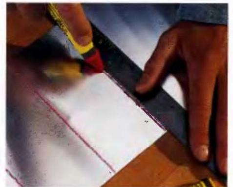
USE A GREASE PENCIL to mark metal, plastic and other materials that can't be marked clearly with a pencil.
