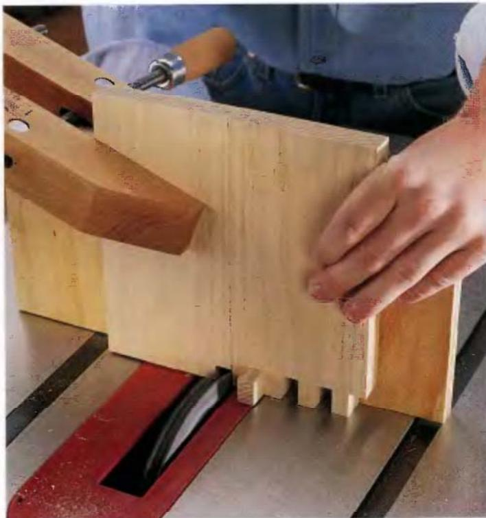
**5** To cut the joints in the mating boards, fit the last notch you cut in the first piece over the pin, then butt the mating piece against the first piece, creating a one-notch offset. Make the first pass on the mating piece. Now remove the first piece, butt the notch in the mating piece against the pin and make the second pass. Continue until all the joints are cut in one end, then flip the board end-for-end and repeat.
