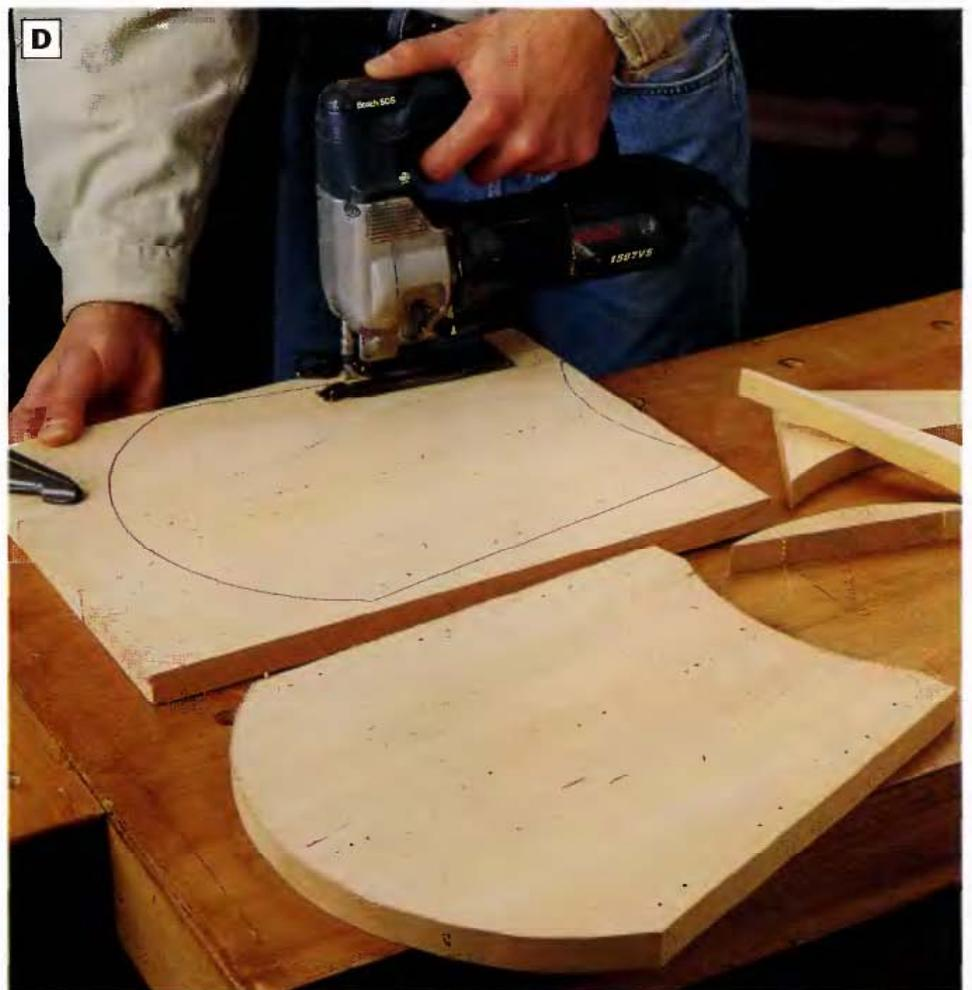
**PHOTO D:** Cut out the end shapes. We used a jig saw, but you could use a band saw or scroll saw instead. Cut along the waste sides of the cutting lines, then smooth the cuts with a file or by sanding with medlum-grit sandpaper.
