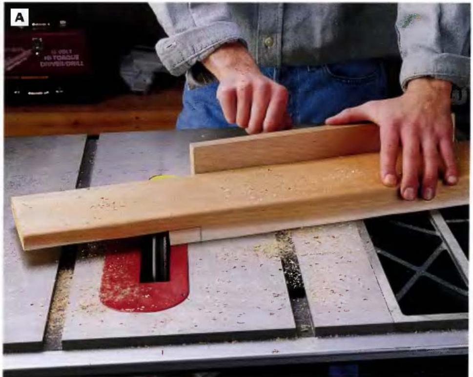
**PHOTO A:** Cut the half-laps in the seat supports and back supports with a dado-blade set, making multiple overlapping passes. The final pass on each board should be right along the marked cutting line. Set the miter gauge to 65°. Making the half-lap joints prior to cutting the contours of the parts simplifies the layout of the contours.
