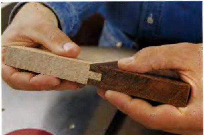
**4** Apply wood glue in the groove, then insert the tongue. The tongue should fit fully in the groove.
