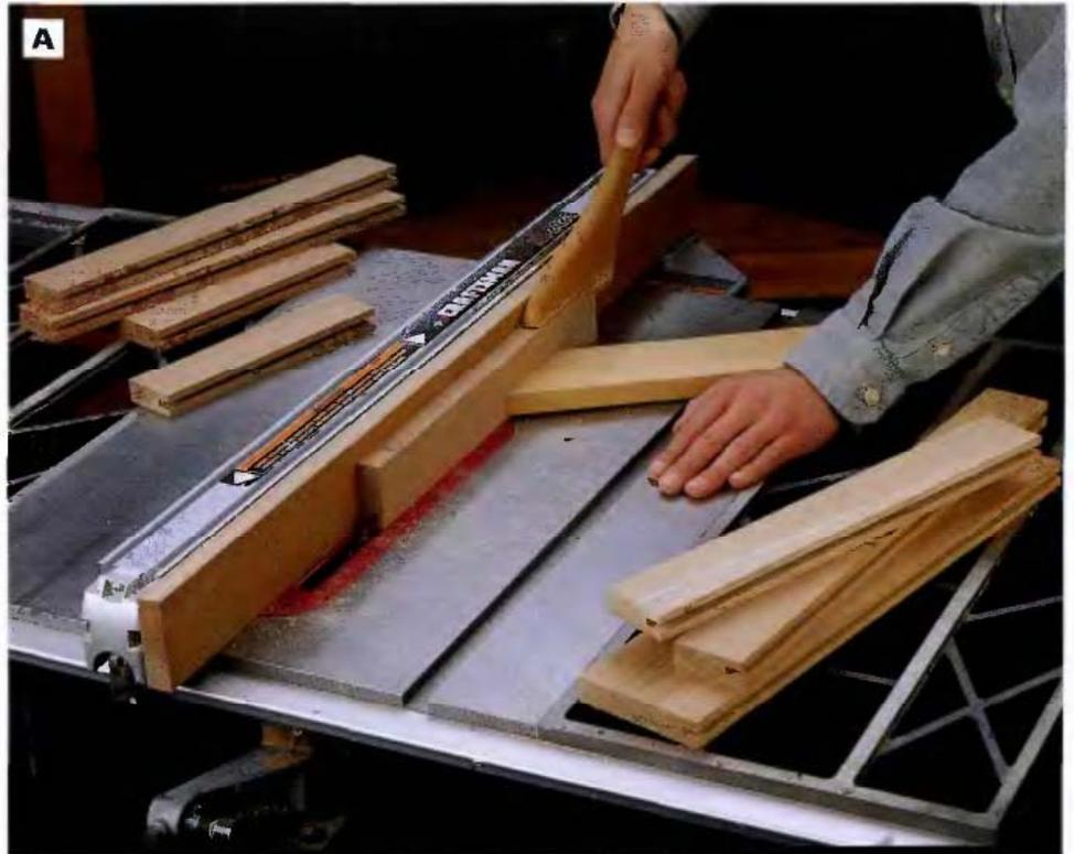
PHOTO A: Cut  $\frac{1}{4}$  ×  $\frac{1}{2}$ -in. grooves in the edges of the side and back rails and stiles. The grooves should be sized so the plywood panels fit into them snugly. Using a featherboard and pushstick, cut the grooves by making multiple passes with the table saw blade.
