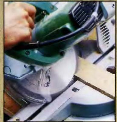
**1** Cut one mating board square, and cut the other at a 45° bevel, using a miter saw. The beveled board should be slightly longer than the finished length.
