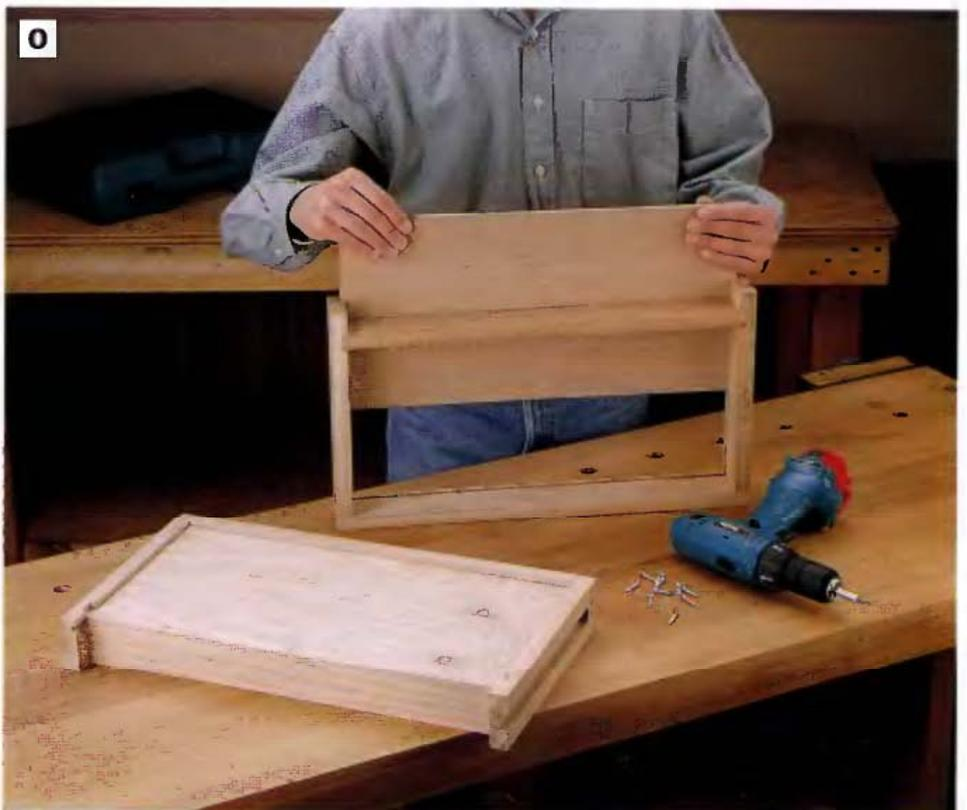
**PHOTO O:** Slide the drawer bottoms into the grooves in the drawer sides and front. Secure the drawer bottoms with three screws driven through the drawer bottom and into the bottom edge of the drawer back. Do not use glue.
