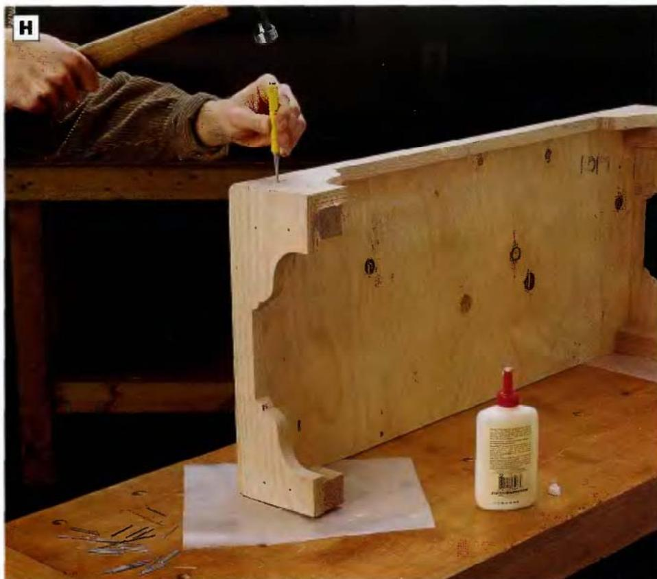
**PHOTO H:** The trim pieces wrap around the base structure, adding decoration and “feet” to the cabinets. Use 4d finish nails and glue to attach the mitered trim pieces. Drill pilot holes for the nails (you can remove the head from a finish nail and chuck it into your drill if you don’t have a drill bit small enough for the job). Set nails with a nailset.
