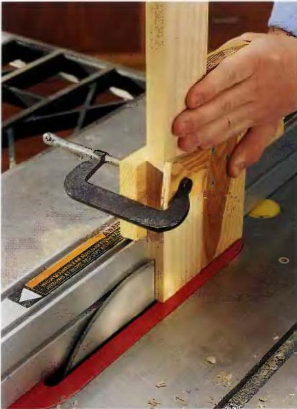
**1** Cut the tongue portion of the lap joint on your table saw, using a tenoning jig to support and guide the workpiece. Set up the saw as if you're cutting a deep rabbet, and begin by making the check cuts.
