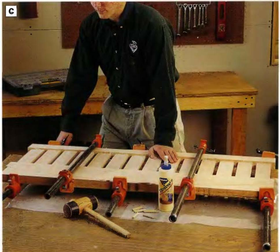
**PHOTO C:** Assemble the upper and lower back rails and back slats with glue and dowels. Clamp the assembly together, using the waste pieces from Step 1 to make clamping the top rail easier. Alternate the clamps above and below the assembly to distribute clamping pressure evenly.
