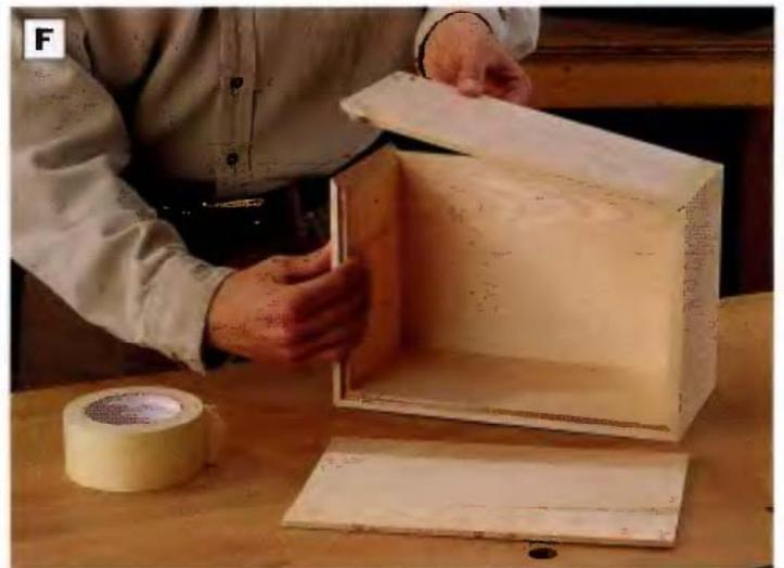
**PHOTO F:** Apply glue to the mitered faces and use tape to hold the corner joints together while the glue sets. Tack the box bottom panel into its rabbet. The lid panel dado gets no glue.
