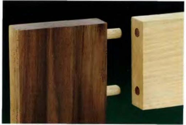
A HIDDEN DOWEL JOINT can be used to reinforce butt joints when assembling face frames or making furniture. The dowels strengthen the joint, and help you align the parts. For best results, use a dowel jig or dowel points for guidance when drilling the dowel holes.
