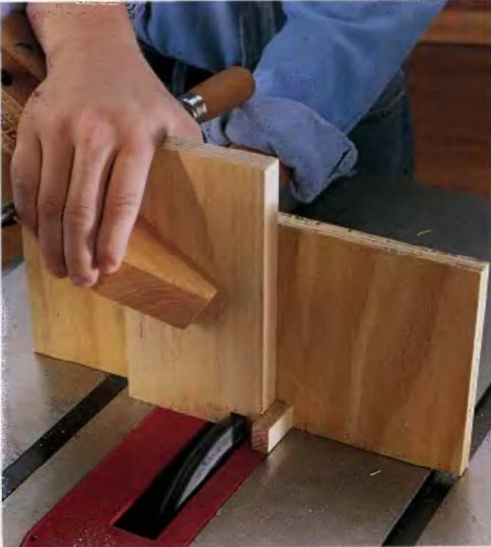
**3** With the pin spacer inserted in the fence slot and the fence in position, butt the first workpiece against the strip and make the first pass. You can hold the workpiece in place by hand or clamp it to make the cut. After the workpiece and fence clear the blade, shut off the saw and back the workpiece off.
