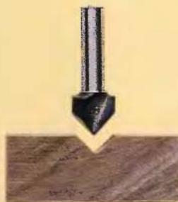
**VEINING (V-GROOVE) BIT.** Used for carving, lettering and cutting decorative V-shaped veins. Most are 90° cutting angle, but 45° and 60° bits can be found. Available sizes: 1/4, 3/8, 1/2, 5/8, 3/4 in.; 1/2 in. shank only: 15/16, 1, 1 1/4, 1 1/2, 2 in.
