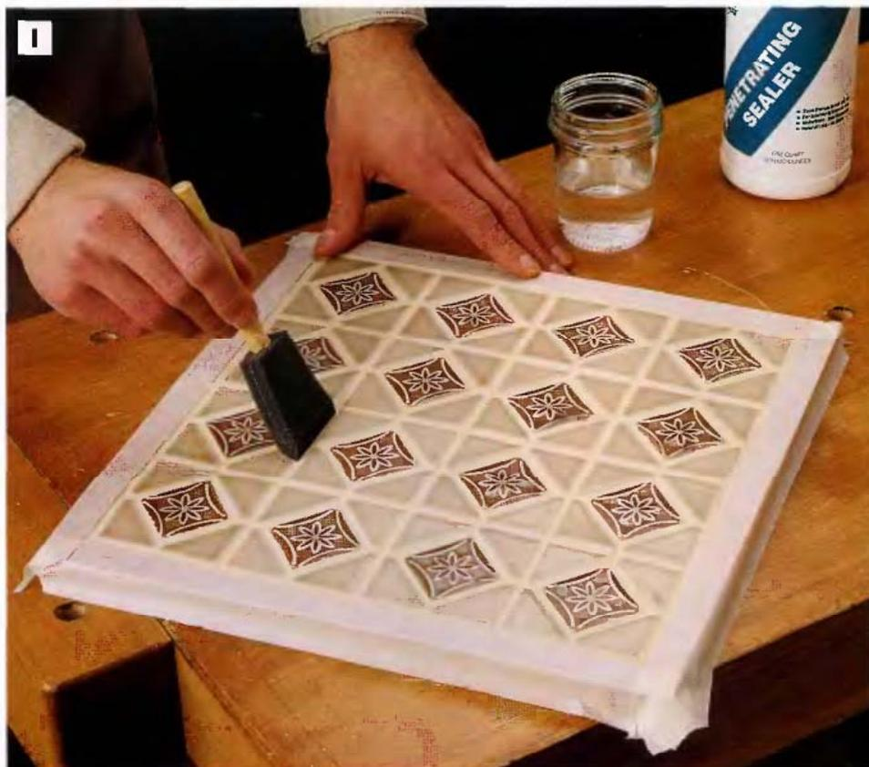
**PHOTO I:** Seal unglazed tile and grout joints with penetrating sealer. Use a disposable foam brush to apply the sealer. Because a plant stand is likely to be exposed to a considerable amount of moisture, sealer is important to protect the plant stand top and to help inhibit mildew and other forms of discoloration that can affect the grout.
