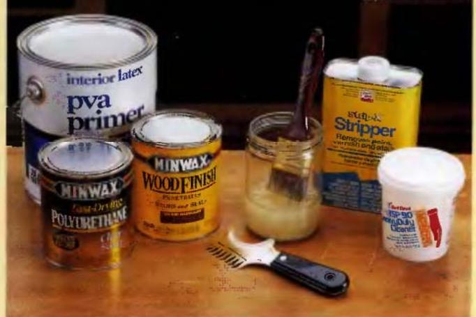
(tsp) solution. Use a brush comb to help clean and condition the bristles. For brushes that are crusted with other materials, try soaking them in paint and varnish stripper to dissolve the gunk, then rinse with tsp and comb. If you know the exact type of solvent used for the product that has dried, try soaking the brush in that product (for example, lacquer thinner) before opting to use stripper.
