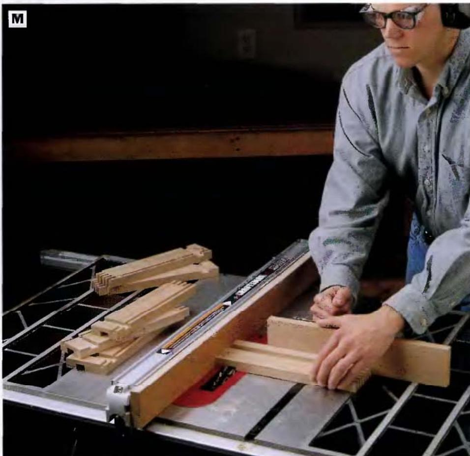
**PHOTO M:** Cut the drawer back dados on the table saw with a dado blade, miter gauge, and rip fence. Push the stock across the blades carefully to avoid binding the workpiece between the blades and the rip fence. Remove the stock after it has cleared the blades.
