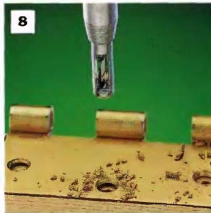
**1. Twist bit** will bore through angle iron, flat iron or sheet metal and can be used for rough drilling in wood and other materials. Twist bits are available in a wider range of diameters than any other bit type.
