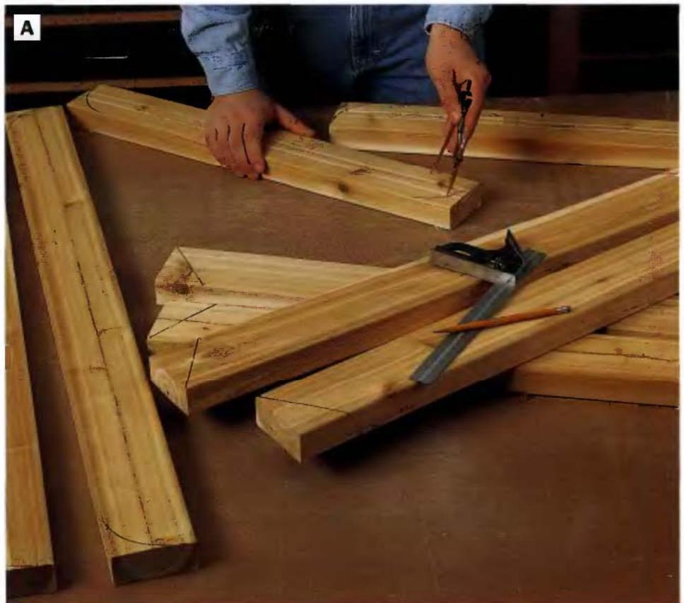
**PHOTO A:** Lay out the legs and stringers. Scribe the curved end of the legs and the curves on the stringers with a compass, set to the radii given in the technical drawings on page 300.
