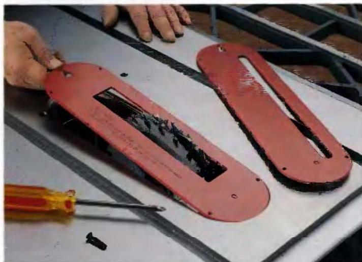
**1** Set the cutting width of your dado blade by adding chippers and spacers between the two blades. Mount the set on your table saw arbor. When mounted in a table saw, dado-blade sets require a saw throat plate with an extra-wide opening.
