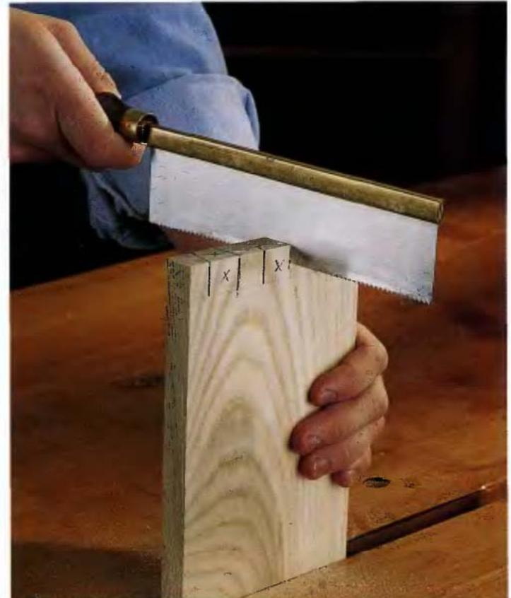
**5** Use a tenon saw, also called a dovetail saw, to cut the shoulders of the pins. Split the lines with the saw, favoring the waste side. Cut down to the scribed lines, but do not cut below the lines or the kerf cut will show when the joint is assembled.
