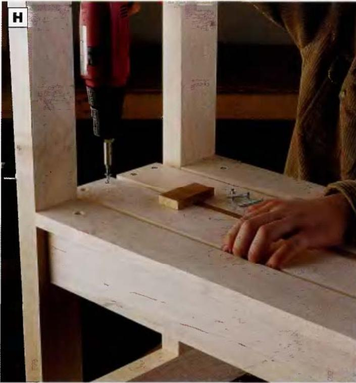
**PHOTO H:** Screw the inner and outer slats to the stretchers and cross braces to create a storage shelf.
