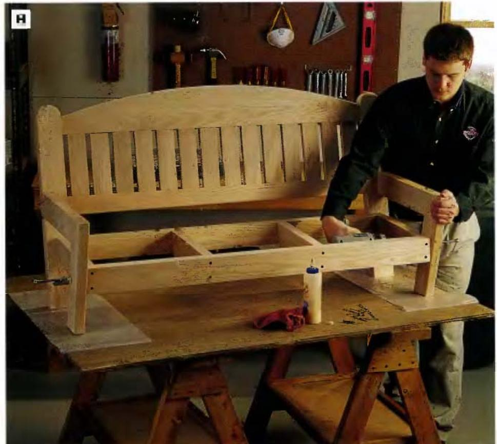
**PHOTO H:** Fasten the arm assemblies to the bench by driving screws through the back stiles and into the arm supports. Screw from inside the bench to attach the end bench struts to the legs as well. Clamp the arm assemblies in place first, to make installing the assemblies easier.
