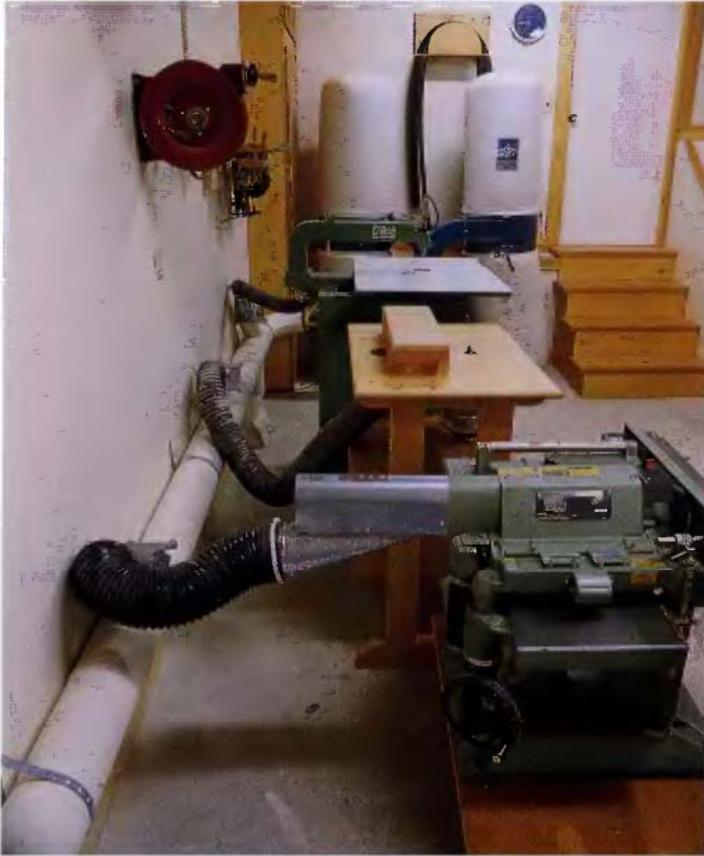
THE TWO-STAGE DUST COLLECTOR in the background of this workshop photo is connected to all of the stationary power tools in the shop with dedicated 4-in. or larger hoses mounted to the walls and positioned to be out of the way when work is taking place.
