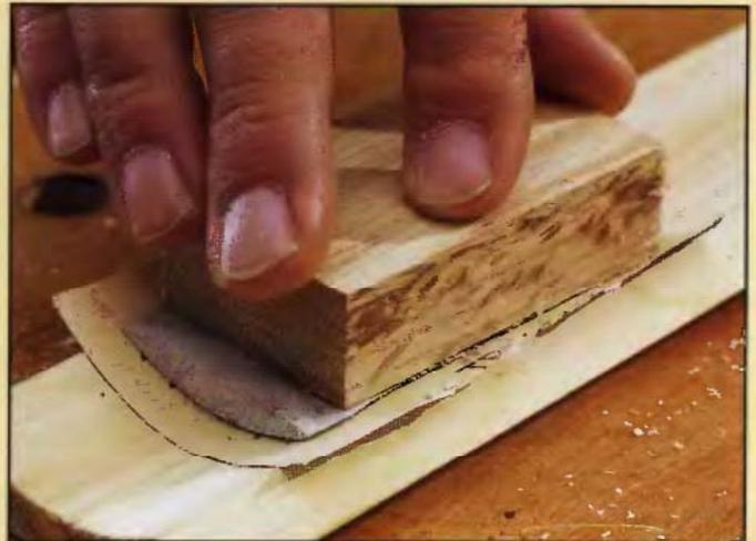
**2** Remove the molded auto body filler and hot-glue a block of wood to the flat face to give the sanding block greater rigidity and durability. Wrap a piece of sandpaper around the shaped face and start sanding. Note: This technique also works with convex sanding profiles.
