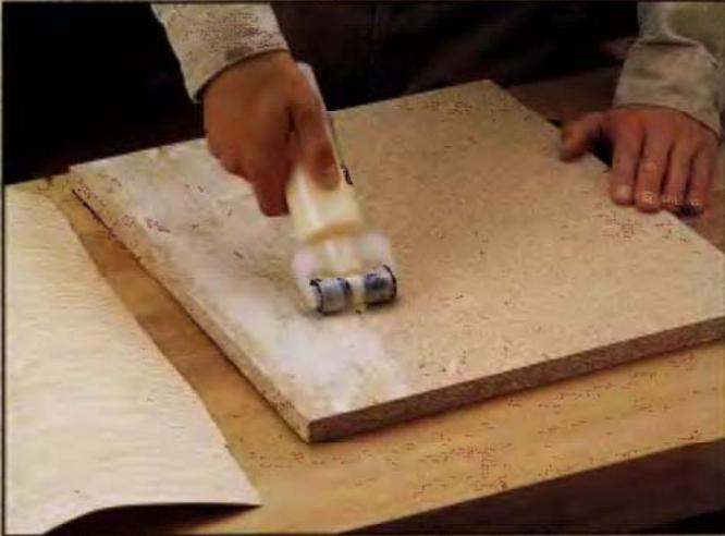
A **GLUE ROLLER** is used to apply an extremely even coating of glue on large, broad surfaces, such as when applying veneer. Once the hopper is loaded with glue, it will dispense glue over the roller at an even rate when the surface is rolled.
