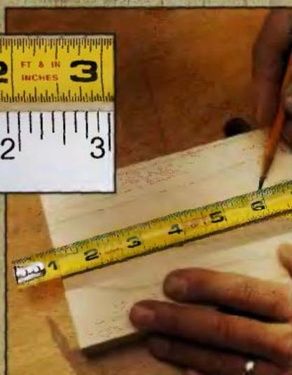
**USING THE END HOOK** as a starting point when taking measurements with a tape measure can be unreliable, as illustrated by the photo above.
