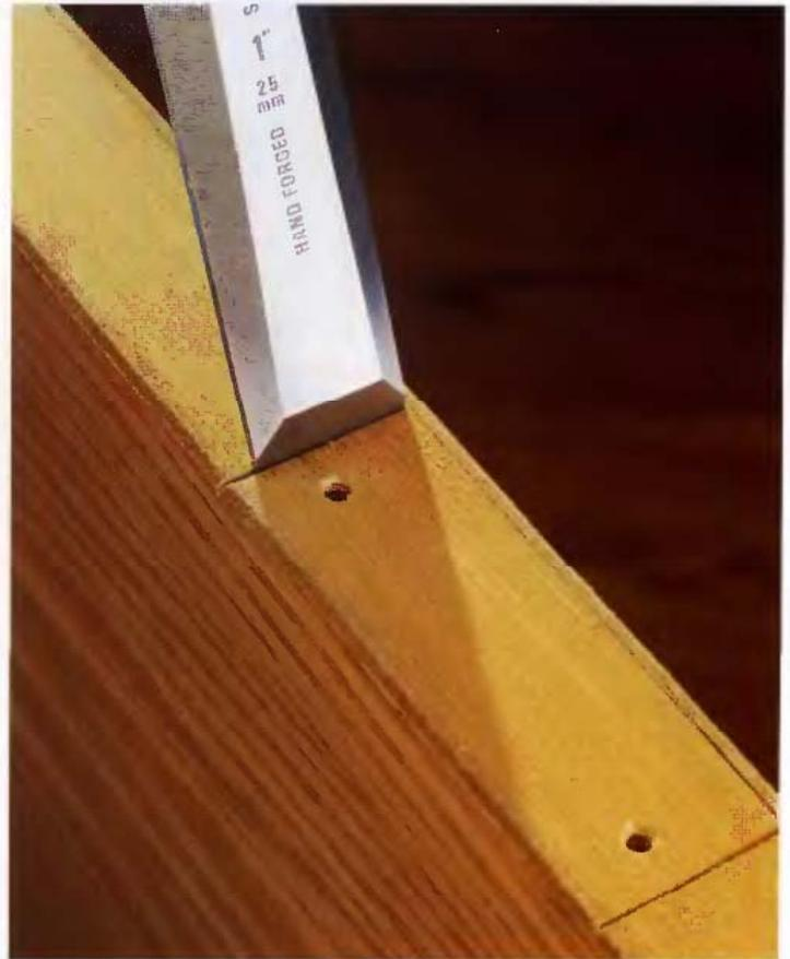
**2** Choose a chisel that's close to the same width as the mortise. With the beveled side of the chisel facing toward the mortise, tap the butt of the chisel handle with a wood or rubber mallet. Cut into the wood to a depth equal to the thickness of the hinge leaf or strike plate. Cut along all sides of four-sided mortises.
