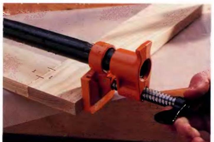
**4** Create all the joints, then clamp the assembly together with pipe clamps or bar clamps. Be sure to use a clamp pad between the wood and the clamp jaws so the jaws don't mar the wood. Do not overtighten the clamps.
