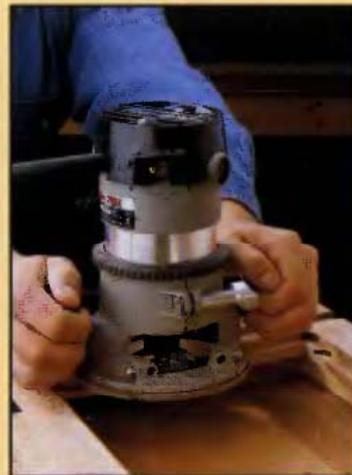
**USE A PILOTED RABBIT BIT** to cut rabbets on the insides of frames or on the outer edges of any workpieces. Make several passes of increasing depth with the router, then square the rabbet corners with a chisel. When profiling an outside edge, clamp scrap blocks at the ends of the workpiece.
