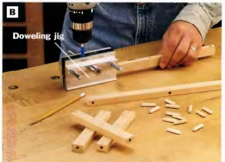
**PHOTO B:** Drill holes in the face frame rails and sides so you can assemble these parts with dowels. A doweling jig ensures that the holes are positioned precisely across each joint and keeps the drill bit straight in relation to the workpiece.
