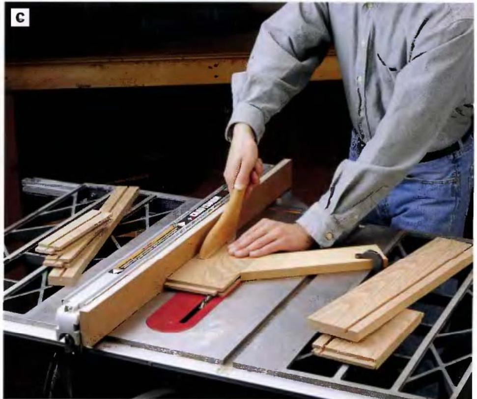
**PHOTO C:** Cut  $\frac{1}{4} \times \frac{3}{8}$ -in. grooves for the upper and lower chest bottoms into the side and front rails. Use a featherboard and pushstick.
