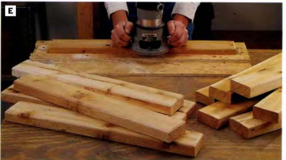
**PHOTO E:** Cut the 19 seat slats to length, and ease the top edges and ends of each slat with a ½-in. roundover bit in the router. We used a plywood jig clamped to the benchtop to “frame” each slat on all sides and hold it steady while routing. This way, the slats require no further clamping.
