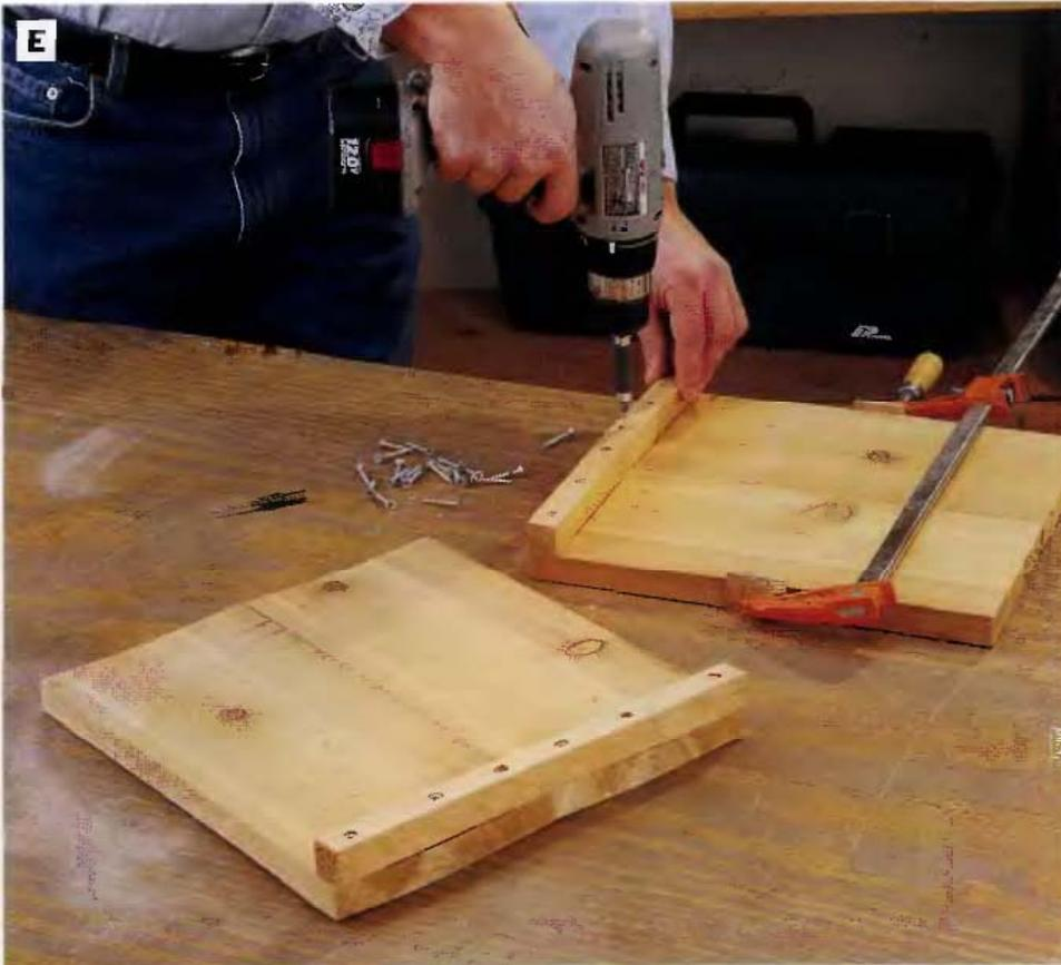
**PHOTO E:** Clamp pairs of 6-in.-wide boards for the end panels and fasten each panel together with a cleat. Use 1 1/4-in. galvanized screws to join the parts. These two cleats are permanent parts of the planter.
