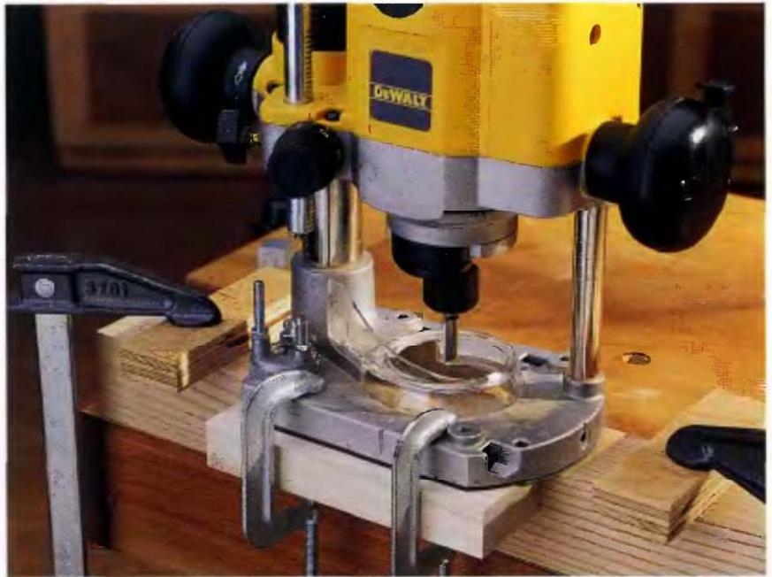
**2** In your plunge router, install a straight bit with a diameter equal to the width of the mortise. Clamp a stop block guide to the router base so the bit aligns with the mortise outline. Set the cutting depth to the depth of the mortise. With the workpiece secured, plunge the bit into the wood and make the mortise cut.
