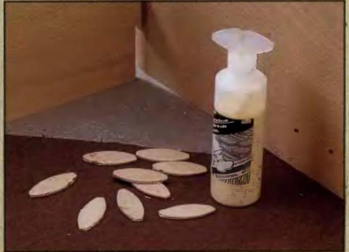
A **SPECIAL GLUE TOOL FOR BISCUITS** can be slipped into a biscuit slot to deliver glue with no spillage or mess.
