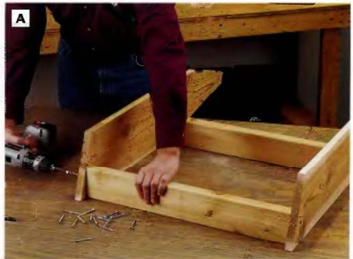
**PHOTO A:** Attach the back legs to the seat stretchers with 2-in. galvanized deck screws. Countersink the screw heads.
