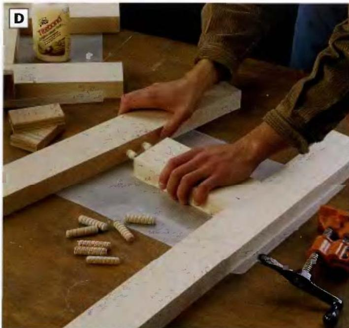
**PHOTO D:** Use fluted,  $\frac{1}{2} \times 2$ -in. dowel pins to reinforce the joints between the legs and the cross braces.
