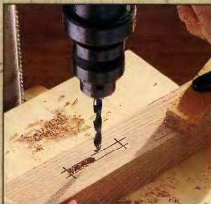
**1** Carefully lay out your mortise using a marking gauge or straightedge. Choose a drill bit the same diameter as the thickness of the mortise ( $\frac{3}{8}$  in. is common), then remove the waste wood from the mortise by drilling overlapping holes using a depth stop.
