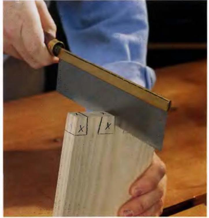
**11** Clamp the board in a vise and use a dovetail saw to make the cuts down to the scribed line. Remove the waste from between the tails with a sharp chisel, the same way you removed the waste from the pin boards. Make the shoulders of the tail board by sawing along the base line to the first tail on each end.
