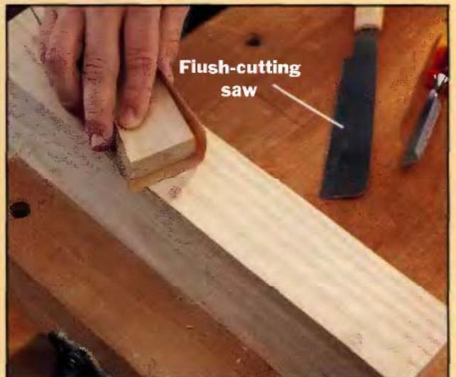
**3** Trim the plug with a chisel, flush-cut saw or rasp, then sand the plug until it's even with the wood surface.
