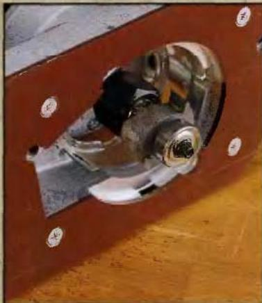
Piloted router bits have a bearing or a fixed spindle that follows the edge of a board as you cut, allowing the cutters to engage the wood and maintain a uniform depth of cut without the need for a straightedge guide. Piloted rabbet bits, like the one shown above, are generally available in sizes that will cut rabbets ranging from  $\frac{1}{4}$  in. to  $\frac{3}{4}$  in. deep.
