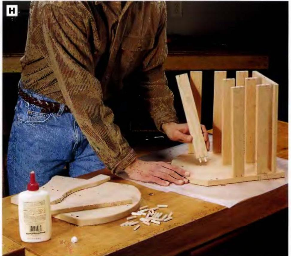
**PHOTO H:** Glue the dowels in the ends of the handle, the slats, and the bottom into the corresponding dowel holes in one side panel. Then immediately glue dowels into the other end panel and set it onto the upright ends of the parts. Align the dowels into their holes and press the assembly together.
