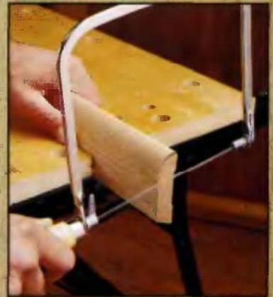
**2** With the square-cut board flush in the corner, use a coping saw to trim the excess wood from the beveled end, leaving an end that's perpendicular but tapers up to follow the profile of the molding.
