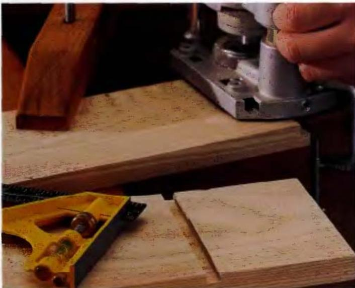
**CUT THE DADOES FIRST** at the joint locations, using a straight router bit or a table saw and dado-blade set. Measure the dados and use the measurements as a guide for cutting rabbets with lips that fit exactly into the dados (in the photo above, a guide block is clamped to the router base and the rabbet cut is made with a straight bit). Make sure the rabbeted ends will not extend more than halfway into the dadoed board.
