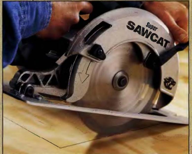
**USE A CIRCULAR SAW:** Place the front edge of the foot against the board, retract the blade guard and hold it in a raised position with your thumb. Turn on the saw and lower the blade into the wood, using the front of the saw foot as a fulcrum. Always wear safety goggles.
