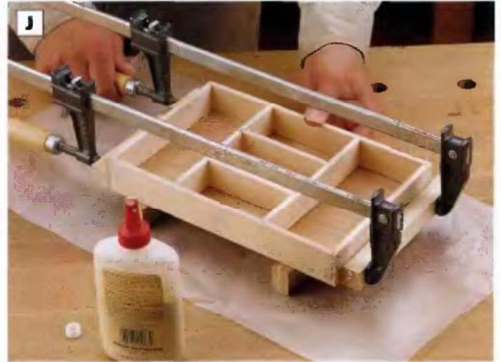
**PHOTO J:** After the tray dividers are assembled, glue up the tray sides and ends and tack the tray bottom in place with brads.
