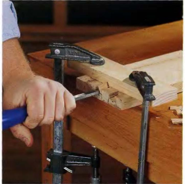
**7** Carefully drive the chisel into the end-grain of the waste area between the pins so the waste wood will break off cleanly at the chisel cut along the baseline.
