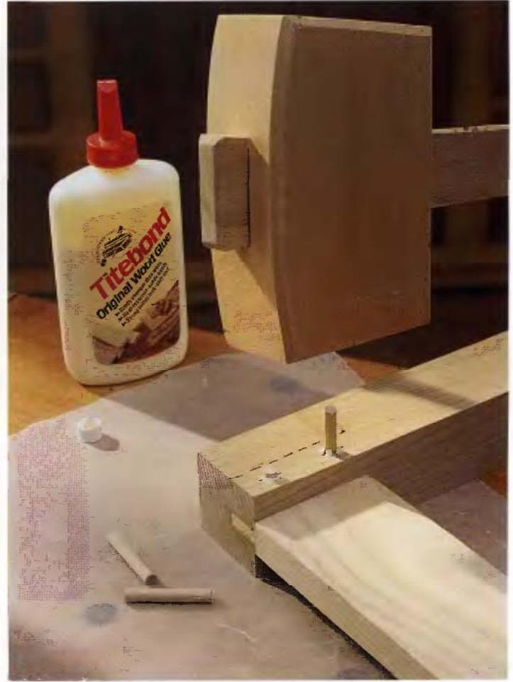
**3** Cut the pins from hardwood dowels, normally of the same species as the workpieces. Tip: For a decorative touch, use dowels made of wood with a naturally contrasting wood tone (for example, maple pins driven into walnut workpieces). Taper the lead tip of the dowel slightly so it will enter the hole more easily. Squeeze a little glue into each hole, then tap the dowel pins home with a wood mallet. Stop tapping when the dowel seats at the bottom of the hole.
