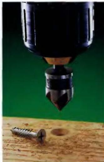
A COUNTERSINK BIT reams out the top of a pilot hole with a bevel that allows the screw head to be recessed.
