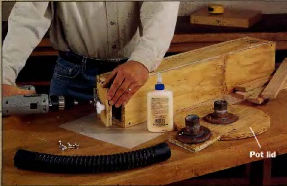
Construct the steamer jig from exterior-grade plywood, moisture-resistant wood glue and galvanized deck screws. Install a hinged door on one end of the steamer box, and drill a 2-in.-dia. hole in the other box end and the plywood pot lid for installing a length of heat-resistant or automotive radiator hose. Attach the hose to the steamer box and pot lid. We used metal fittings and threaded pipe for making these hose connections.
