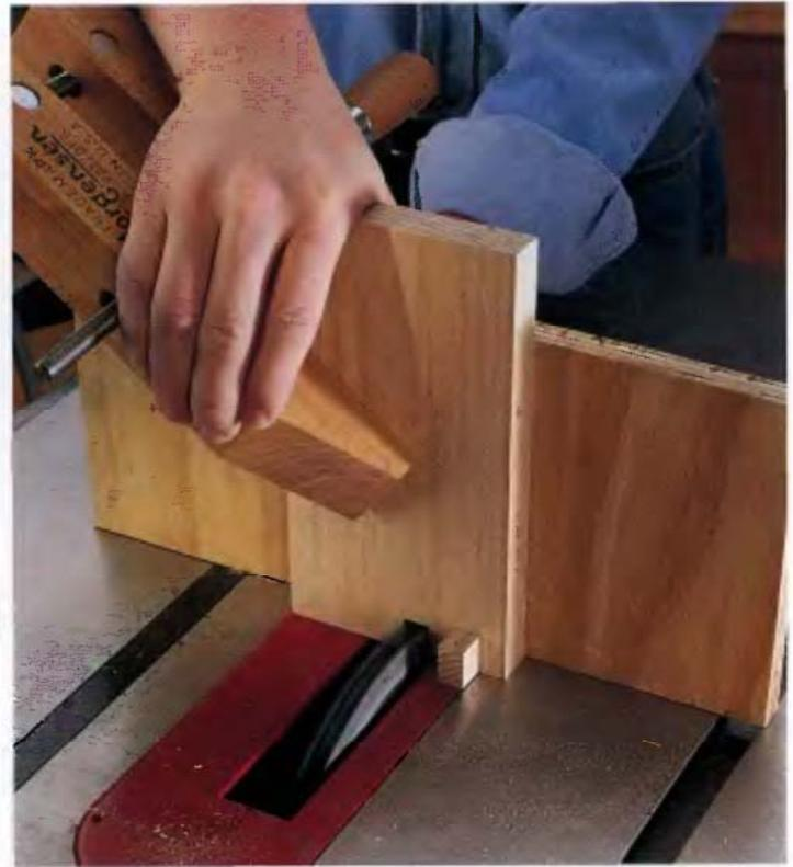
**4** Reposition the workpiece by placing the slot you just cut over the pin space, then make the next cut. Continue in this manner until all the joints in that board are cut. Flip the board end-for-end and cut the fingers on the other end of the board the same way.
