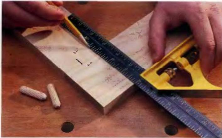
**1** To lay out the dowel joints, butt the two mating parts together, making sure the mating surfaces are flush. Mark the dowel hole locations by drawing a single line across the joint for each dowel. For best results, use at least two evenly spaced dowels at each joint.
