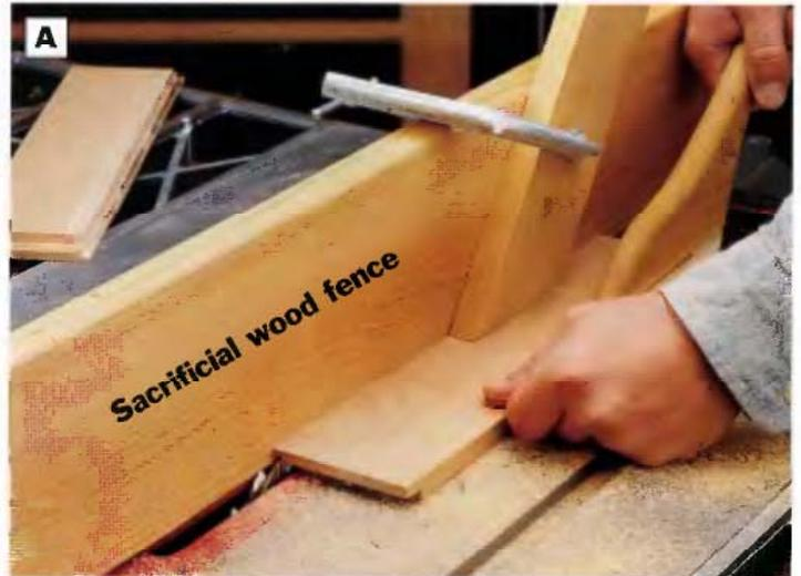
**PHOTO A:** Cut rabbets across the ends and along one long edge of each side piece using a dado blade on the table saw. These rabbets form recesses for the carcass top and bottom, as well as the plywood back panel. Attach a sacrificial wood fence to your saw fence to protect the metal fence from the dado blade.
