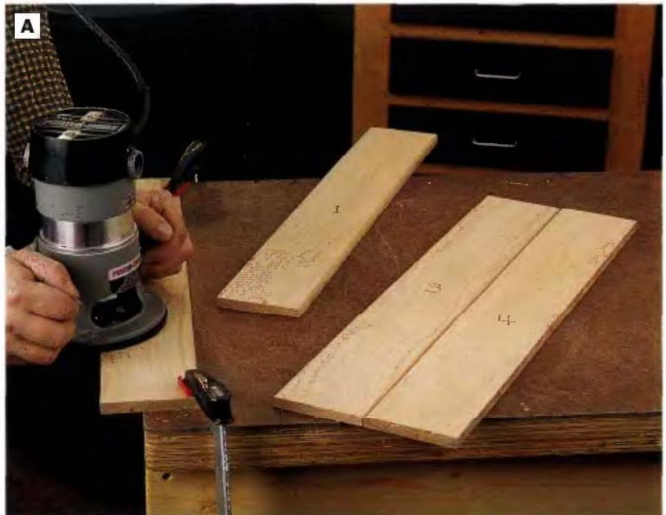
**PHOTO A:** Rout chamfers along the mating edges of the back slats with a piloted chamfering bit set to a cutting depth of <sup>1</sup>/<sub>8</sub> in. It's a good idea to label the slats first so you profile only the edges that will meet once the panel is glued up.
