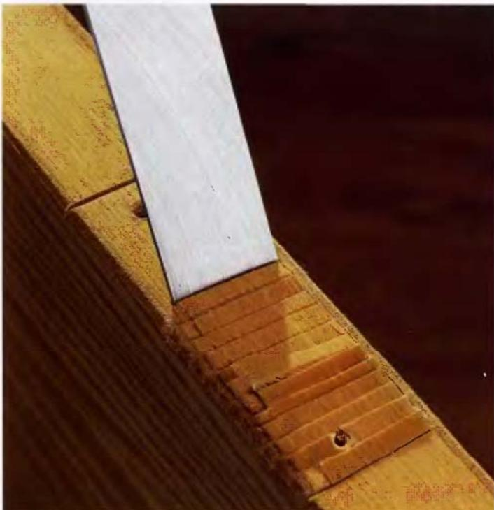
**3** With the beveled edge of the chisel tip flat against the workpiece, make a series of relief cuts in the waste wood area of the mortise. Space the cuts  $\frac{1}{8}$  to  $\frac{1}{4}$  in. apart (make closer cuts in harder woods). The cuts should be equal in depth to the finished depth of the mortise.
