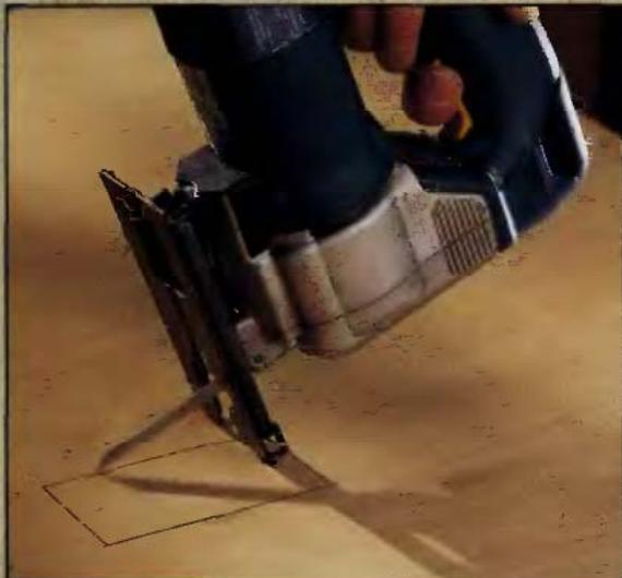
**USE A JIG SAW:** Tip the Jig saw forward on the front edge of its foot. Align the tip of the blade with the cutting line, then turn on the saw and gently but firmly lower the blade into the cutting area. The blade will want to bounce, but by maintaining firm pressure on the front of the foot you can keep it under control until it enters the wood.
