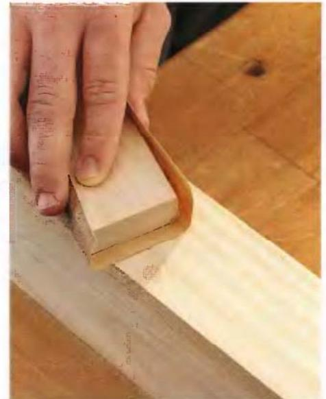
**3** After the glue has dried, trim the plug flush with the wood surface using a flush-cutting saw (See photo, above left). Take care not to mar the surrounding wood surface. Sand the plug smooth.
