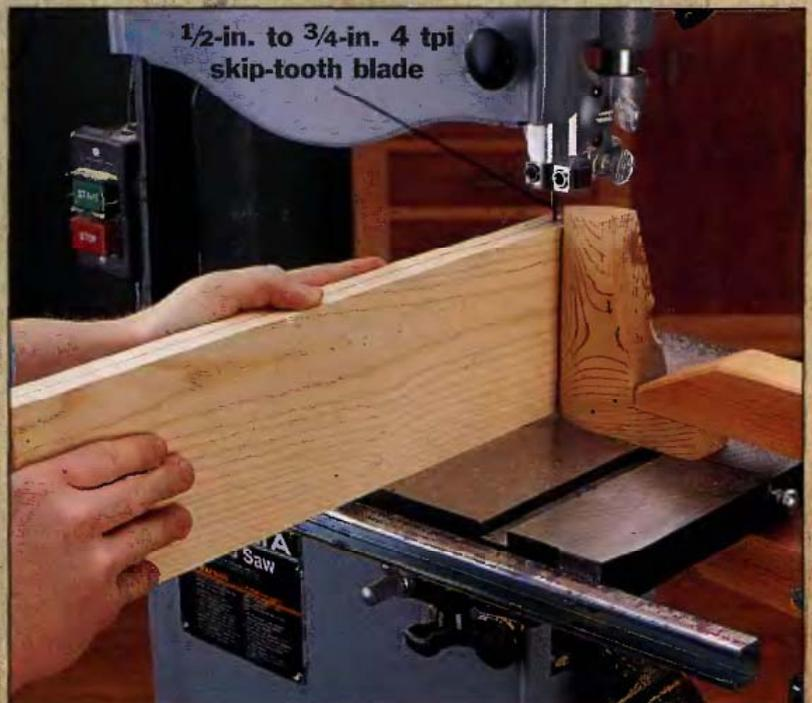
**RESAWING THICK LUMBER** into thinner strips for woodworking is a job best accomplished with a band saw. The simplest method is to attach a fence to the band saw table, parallel to the blade, and feed the stock through as you would when rip-cutting on a band saw. The downside to this method is that the saw blade tends to travel, following the grain of the wood, and resulting in an uneven cut that requires quite a bit of surface planing. One way to minimize the unevenness of the resaw cut is
