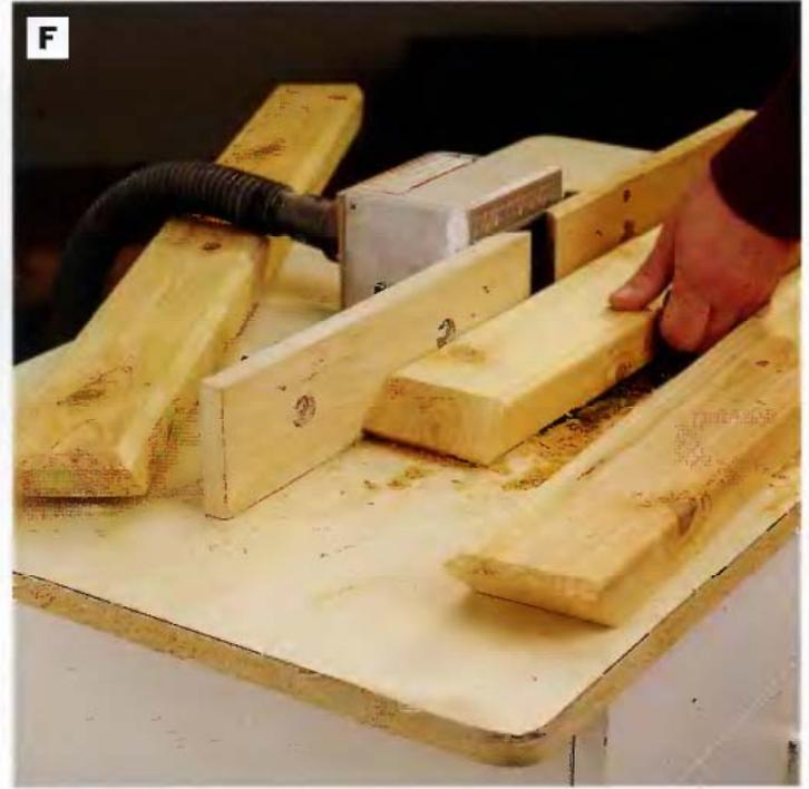
**PHOTO F:** The bottom edge and both ends of each apron piece are chamfered. Make these cuts at the router table, using a piloted chamfering bit set to a height of  $\frac{3}{8}$  in.
