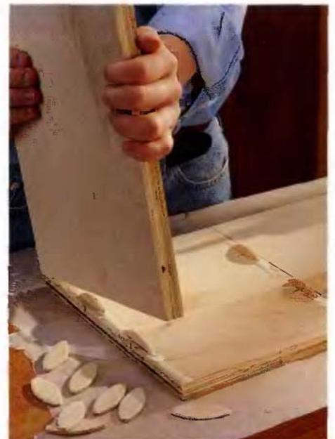
**3** With all the slots cut, you're ready for assembly. Apply glue in the biscuit slots and on the mating surfaces. Insert all the biscuits into the slots in one workpiece, then slip the mating workpiece into position so the parts butt together cleanly. Clamp the parts together, check for square and adjust the clamps as necessary to square up the joints.
