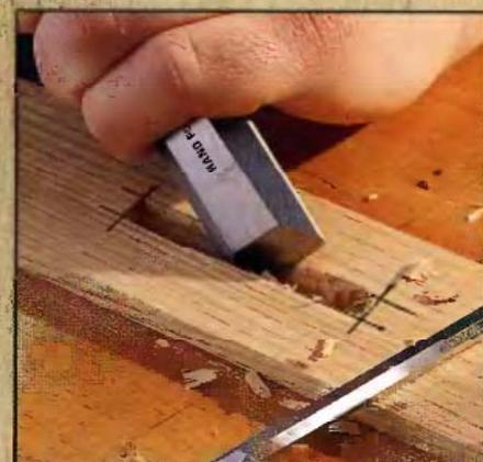
**2** Use a sharp chisel to clean up the sides of the mortise so they’re flat and smooth. Make sure the flat face of the chisel is contacting the wood. Clean up the ends of the mortise with a chisel the same width as the thickness of the mortise.
