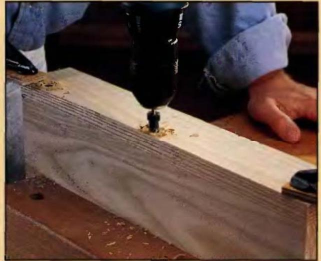
**1** Use a counterbore bit to counterbore the pilot hole for the screw ( $\frac{3}{8}$  in. is the standard counterbore diameter).
