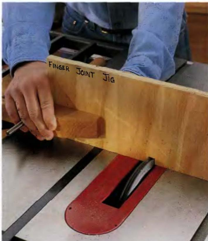
**1** Install a dado-blade set and throat plate in your table saw. Set the cutting width of the dado-set to equal the thickness of the finger pins to be cut. Raise the blade set to cut the full depth of the pins. Clamp an auxiliary fence board to your table saw miter gauge. The board should be about 6 in. wide and at least 18 in. long. Make a pass of the auxiliary fence over the blade, then cut a strip of hardwood to use as a pin to fit in the slot, and glue it into the fence slot.
