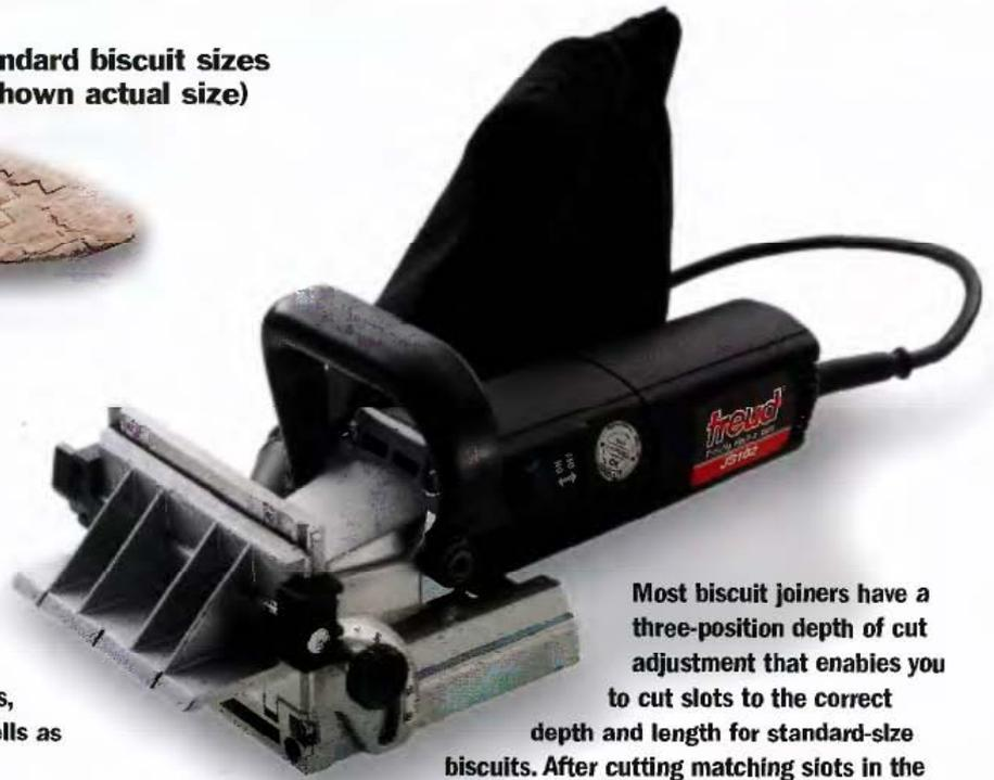
Most biscuit joiners have a three-position depth of cut adjustment that enables you to cut slots to the correct depth and length for standard-size biscuits. After cutting matching slots in the pieces to be joined, you glue the slightly undersized biscuits into the slots.
