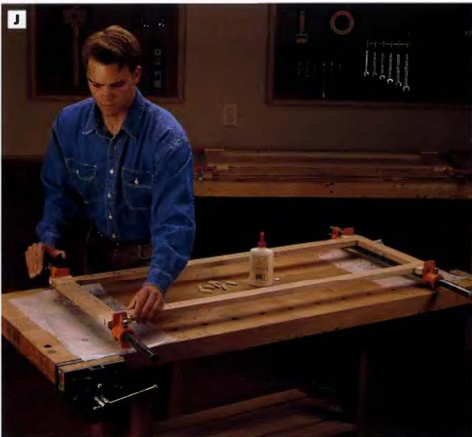
**PHOTO J:** Glue the dowel joints and clamp together the rails and stiles for the face frame, side frames and door.
