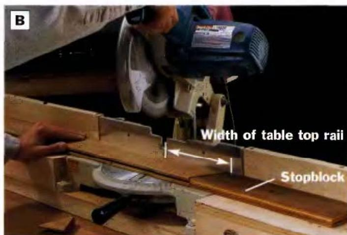
**PHOTO B:** Cut the tabletop rails to length with a  $22\frac{1}{2}^\circ$  angle on each end. Attach an angled stop block to the saw table for consistent cuts.
