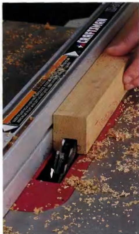
**2** Set the cutting height to the desired dado depth, then adjust the fence so the blade set will start cutting at the shoulder of the planned dado. Make a test cut first, feeding the stock through the blade slowly, with plenty of downward pressure. Use a pushblock when you near the blade. Measure the dado on the scrap and adjust your setup as needed. In harder stock, it's a good idea to make the cut in multiple passes of increasing cutting depth.
