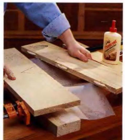
**1** Arrange the jointed boards together to get the most pleasing match of the different grain patterns. This can take some trial and error. **Tip:** alternate the direction of the growth rings at the ends of the boards. This helps keep the panel from cupping. Once you've got all the boards arranged to your satisfaction, draw a "V" across all joints in the panel. Use the legs of the "V" to maintain your alignment as you glue-up the panel.
