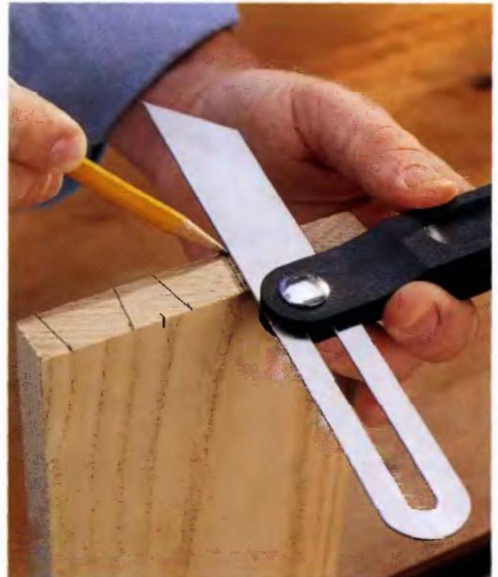
**2** After edge-gluing and cutting the workpieces to size, begin work by laying out the pins. Use the drawing labeled "Pin/tail layout" to lay out the pins on the end of the board with a pencil and the adjustable square.
