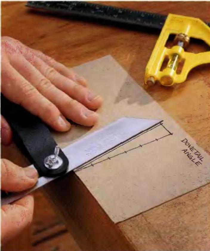
**1** Draw the dovetail pin angle and use it to set the angle on a sliding T-bevel that you can use to mark the pins on the ends of the pin boards. Make a scale drawing of a dovetail pin and use it to set a sliding T-bevel for marking the layout lines for the pins. A standard angle is  $80^\circ$ , which equals a 1:6 ratio of slope to pin depth.
