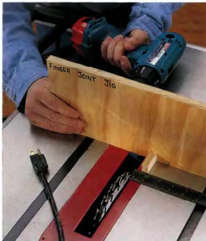
**2** Reset the auxiliary fence by moving it a distance equal to the thickness of one pin to the outside edge of the blade set. Recamp or screw the fence to the miter gauge.
