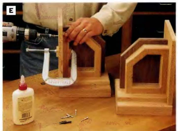
**PHOTO E:** Position the front plates on top of the bases, clamp them in place and attach them to the frame/divider assemblies with glue and four 1 1/4-in. flathead wood screws.
