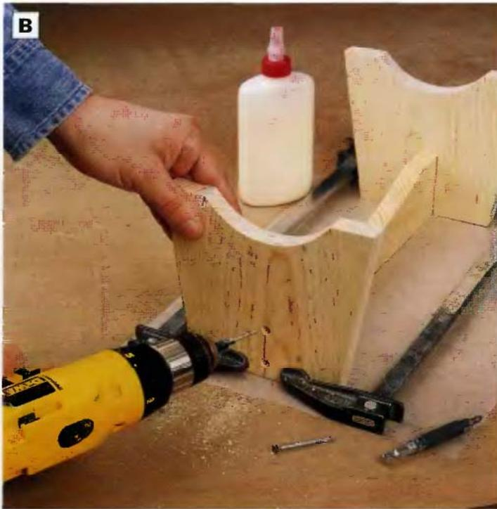
**PHOTO B:** Glue and clamp the stretcher between the legs so the top ends and edges of the parts are flush. Fasten the parts with countersunk 2-in. flathead wood screws.
