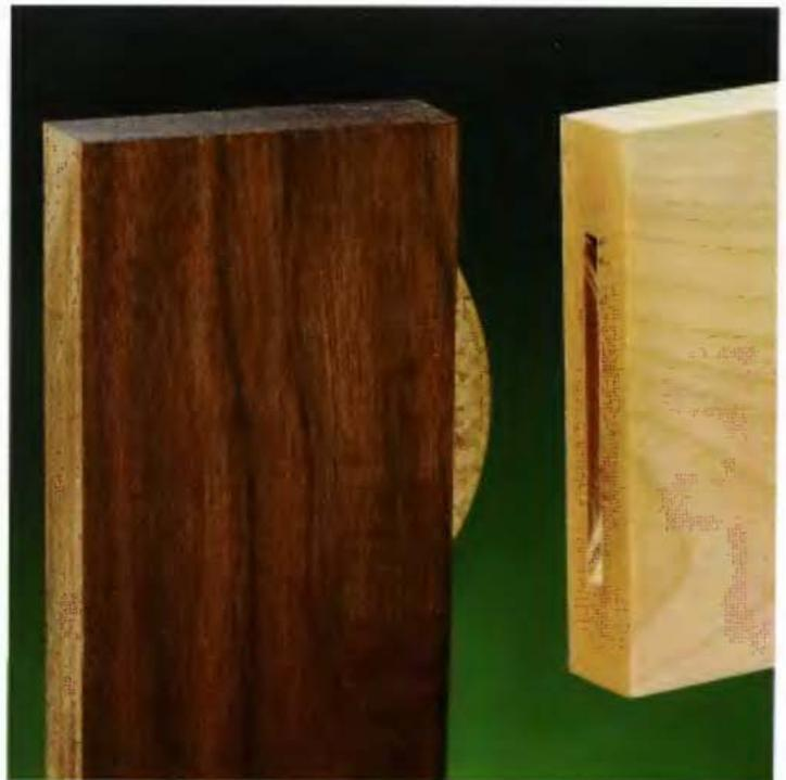
A **BISCUIT JOINT** is a reinforced butt joint used mostly in casework projects. Made with the use of a biscuit joiner (also called a plate joiner) biscuit joints are quick and easy to make. In addition to reinforcing butt joints in face frames, they are frequently employed to help align and reinforce joints when edge-gluing panels from narrower stock or butting sheet goods together to form a carcass.
