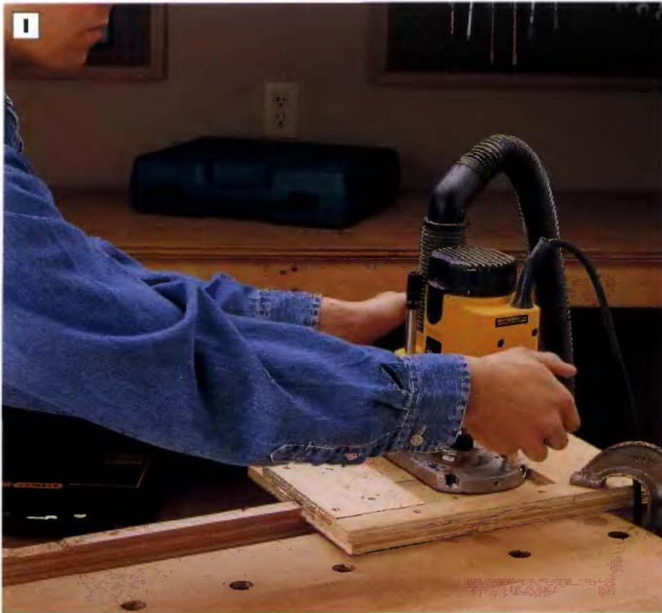
**PHOTO I:** To rout the hinge mortises, clamp a face frame stile on-edge in your bench vise. Clamp a shop-made hinge-mortising jig to the bench so it straddles the stile edge. Run the router around the inside of the jig frame to cut the hinge mortise.
