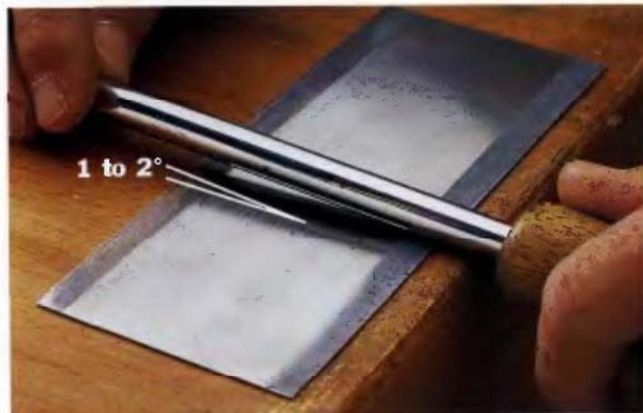
**3** With the scraper lying flat on a work surface, rub across the edges of the scraper with a burnishing tool held at a very slight angle. If you don't have a burnishing tool, any piece of round hardened steel (like the top of a chisel shank) will do. The edge of the scraper should be set back just slightly from the edge of the work surface to prevent you from burnishing at an angle that's too steep.
