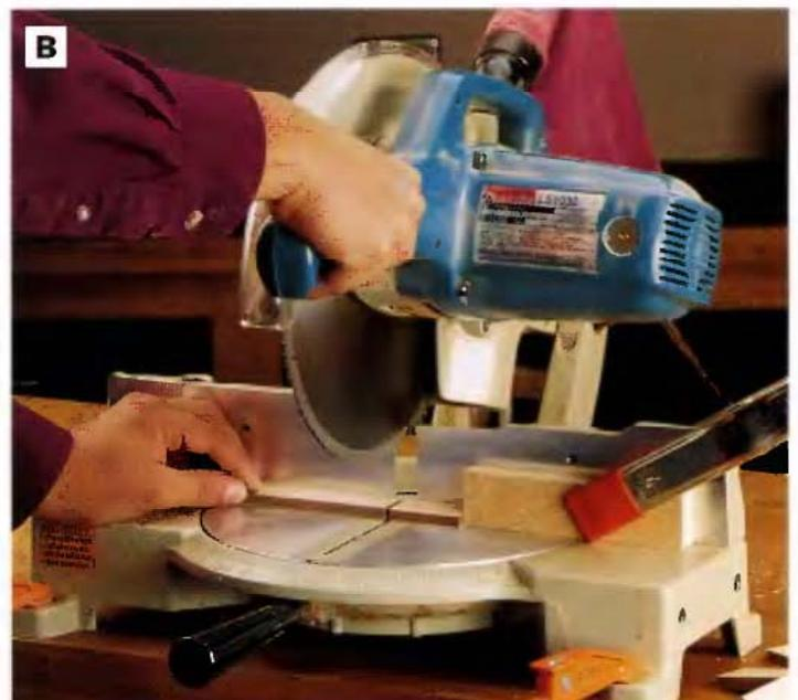
**PHOTO B:** Crosscut the laminated strips into individual domino tiles using a stopblock clamped to the fence of a power miter saw. Set the block 2 in. from the blade, and cut the dominoes one after the next.
