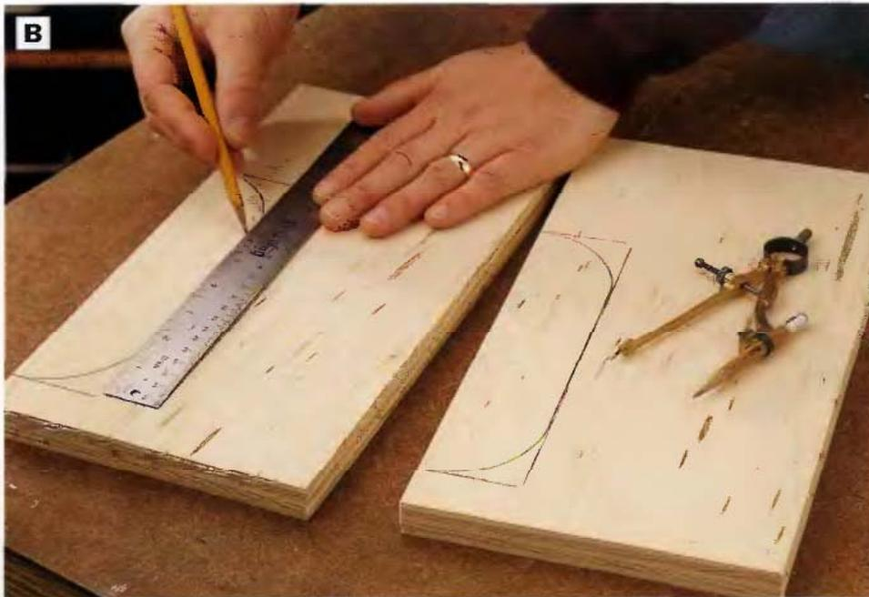
**PHOTO B:** Lay out the curves on the bench legs. Set your compass to draw a 2-in. radius to draw the arcs. Connect the layout lines with a straightedge.
