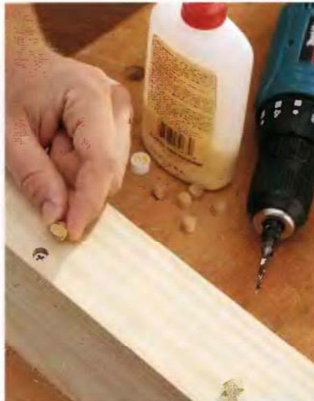
**2** After the screw is driven, apply wood glue to the end of a screw plug. Set the plug into the counterbore hole with a wood mallet. For contrast, the grain in the plug should be perpendicular to the workpiece grain. For concealment, align the patterns.
