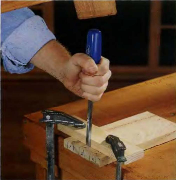
**6** Score along the scribed baseline with a chisel to prevent tearout when you remove the waste around the pins. To ensure a straight scored line, clamp a block of wood next to the scribed line and use it as a chisel guide.
