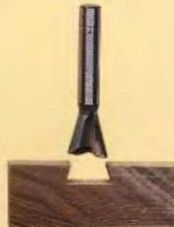
**DOVETAIL BIT.** Used to cut dovetail joints, generally with a dovetail jig. Angles of flutes vary between 7 and 14°. Available sizes: 1/4, 5/16, 3/8, 1/2, 5/8, 11/16, 3/4 in.; 1/2 in. shank only: 13/16, 1 in.
