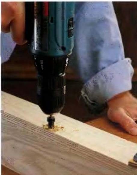
**1** Drill a counterbored pilot hole using a counterboring bit or by drilling a pilot hole, then counterboring for the screw shank and the screw head, according to the dimensions in the chart above.
