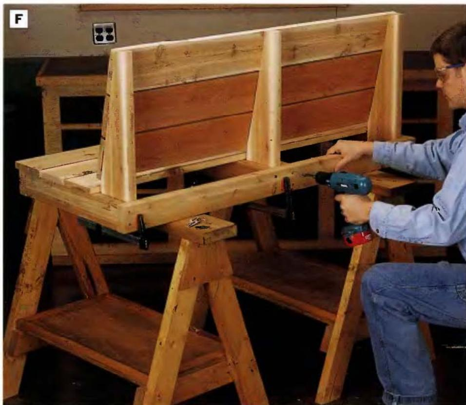
PHOTO F: Fasten the bench back to the seat by slipping the back supports inside the seat frame and between the stretchers, then screwing through the seat frame back and stretchers into the back supports.
