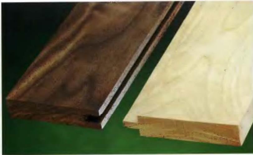
**TONGUE-AND-GROOVE JOINTS** are fashioned by cutting a centered tongue in the edge or end of one board that fits into a centered dado or groove on the mating workpiece. By centering the tongue and fitting it into a centered dado or groove, the shoulders on the tongue side of the joint completely hide the slot made by the dado or groove—a real advantage for concealing the slot-side of the joint.
