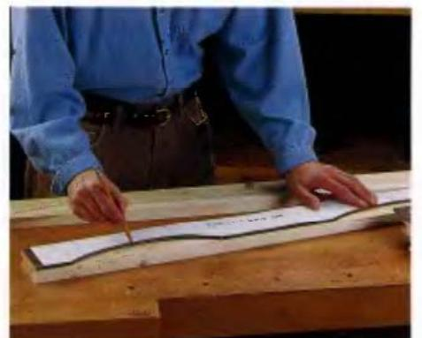
MAKE A STURDY TEMPLATE from hardboard or another durable material when making multiple parts with the same profile.
