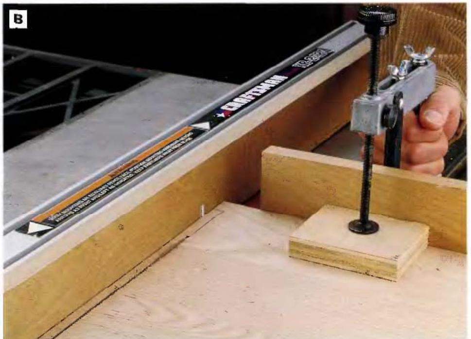
PHOTO B: Cut notches in the ends of the upper cabinet's top and bottom panels. Stop the cuts before the blade cuts past the end line of the cuts, and finish the cuts with a hand saw or jig saw. The notches create a  $\frac{3}{8} \times \frac{3}{4}$ -in. tab that fits over the front edge the side panel on the upper cabinet, creating a recess below for the cabinet door frames.
