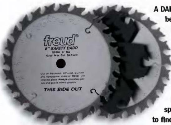
A DADO BLADE SET can be mounted on a table saw and adjusted to cut dados up to  $\frac{7}{8}$  in. wide. The blade sets consist of a pair of circular blades that sandwich toothed chippers. Thin plastic spacers can be inserted to fine-tune the width.
