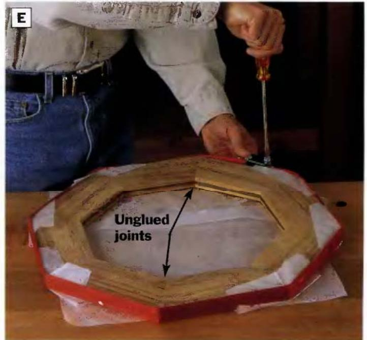
**PHOTO E:** Clamp the top rail assembly with a strap clamp, leaving two opposite joints unglued. Use wax paper around the glued corners to keep the strap from bonding to the wood.
