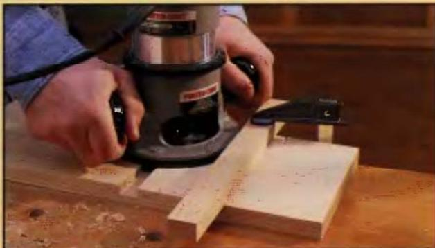
**STRAIGHT BIT AND CUTTING GUIDE.** A router guide is needed to make a dado or plow with a straight router bit. The simplest guide is a plain, straight board clamped to the workpiece the correct distance from the cutting line.
