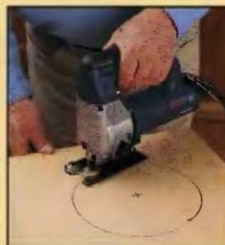
**KEEP PRESSURE DIRECTLY ABOVE THE BLADE.** Whether you're using a top-handle saw, like the one above, or a barrel grip saw, hold the tool so your hand is forward and directly above the blade area. Take care not to force the saw: the blade will break or deflect from the cut line.
