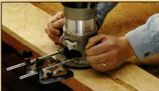
**ROUTER EDGE GUIDE.** For rough work, sliding attachments that fit onto the router base may be used as a guide. Select a bit with a diameter equal to the desired width of the dado. Make the cut in multiple passes of increasing depth, moving the router left to right.
