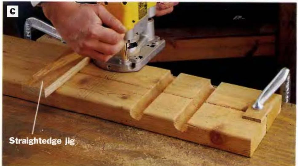
**PHOTO C:** Gang-rout notches in the back supports to ensure that the notches will line up perfectly on both pieces. Use a ¾-in. core box bit, and cut the notches in several passes of increasing depth. We clamped a short T-square style straightedge jig to guide the router when cutting.
