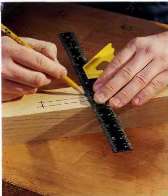
**1** Lay out an outline for the mortise on the workpiece using a pencil and combination square. If you need to make multiple mortises the same width and in alignment, use a marking gauge.
