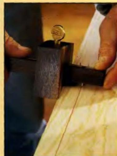
**WOODWORKING:** The most accurate parallel lines can be drawn with a marking gauge. Measure the distance and firmly glide the tool the length of the cut.
