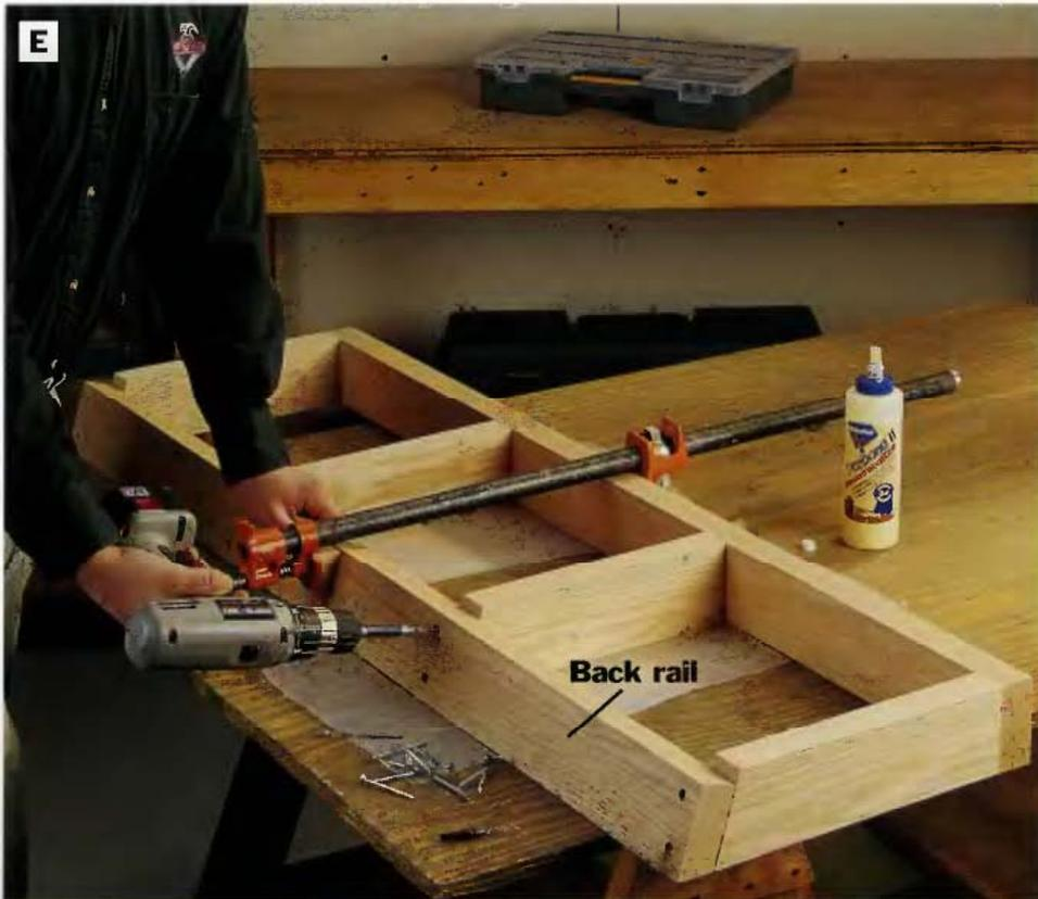
**PHOTO E:** Build the bench frame by installing four struts between the front and back bench rails with glue and screws. In this photo, the bench frame is upside down. Notice that the beveled edge of the back rail lines up with the edges of the struts, leaving an offset on the other edge.
