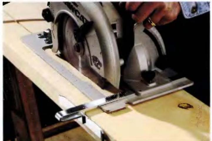
**ADJUSTABLE RIPPING FENCE:** Most circular saws come with an adjustable ripping fence that attaches to the foot of the saw. The fence rides along the edge of the board to guide the saw so it cuts a line parallel to the board edge. These accessories are fine for rip cuts that don't demand a high level of accuracy.
