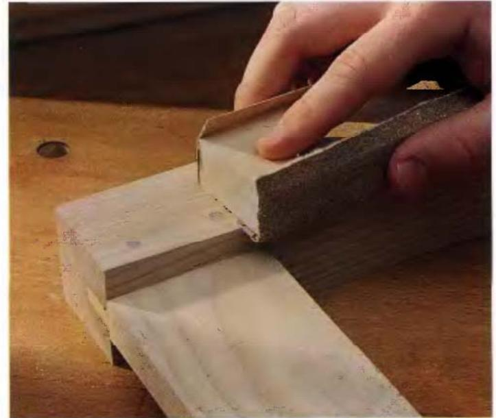
**5** Finally, remove any excess glue with a scraper and sand the surface smooth with sandpaper and a wooden sanding block.
