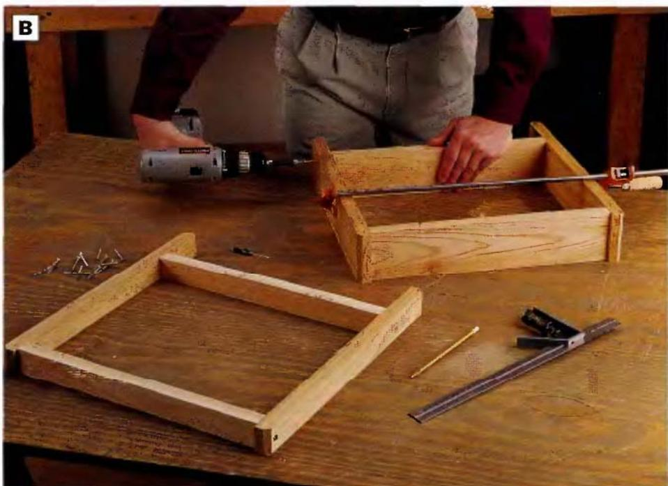
**PHOTO B:** Build an upper and lower frame for each chair. Note that the end pieces of each frame are inset  $\frac{3}{8}$  in. and  $3\frac{1}{8}$  in. from the ends of the side pieces. Clamp the frame parts together, and drive 2-in. galvanized deck screws through the sides and into the ends to make the frames.
