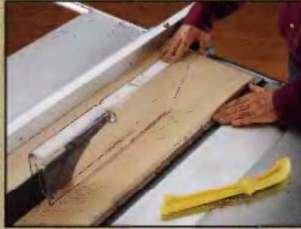
**2** Continue feeding the workpiece through the blade with your right hand as the end of the board approaches the front edge of the saw table. Switch to a pushstick in your right hand if necessary. Keep your left hand on the infeed side of the blade at all times.
