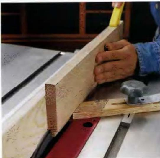
**2** On the uncut mating board, remove the waste wood on one side of the tongue area. Any rabbet-cutting technique may be used with either a standard blade or a dado blade.
