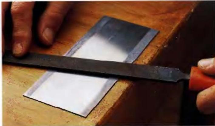
**1** File down any traces of the old burrs on all edges of the cabinet scraper, using a fine single-cut metal file. Don't get too aggressive with the file—it doesn't take much power to remove a fine burr.
