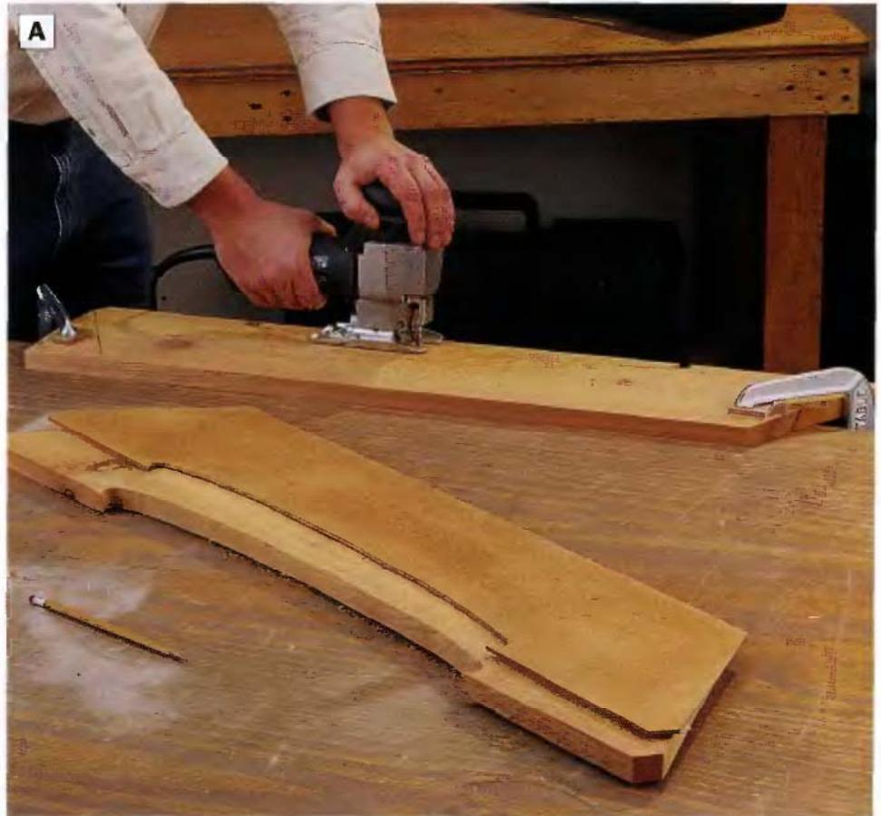
**PHOTO A:** Lay out and cut a template for making the sides of the railing planter, then use this template to draw the shapes on the side workpieces. Cut out the shapes with a jig saw.
