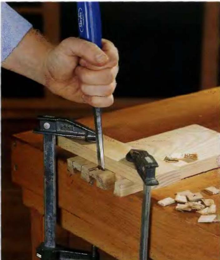
**8** Remove waste in half the area, then flip the board over and continue removing waste from the other side. The beveled face of the chisel should face toward the ends of the dovetails, with the flat face contacting the guide board. When all the waste is removed, clean up the cuts carefully with a smoothing file.
