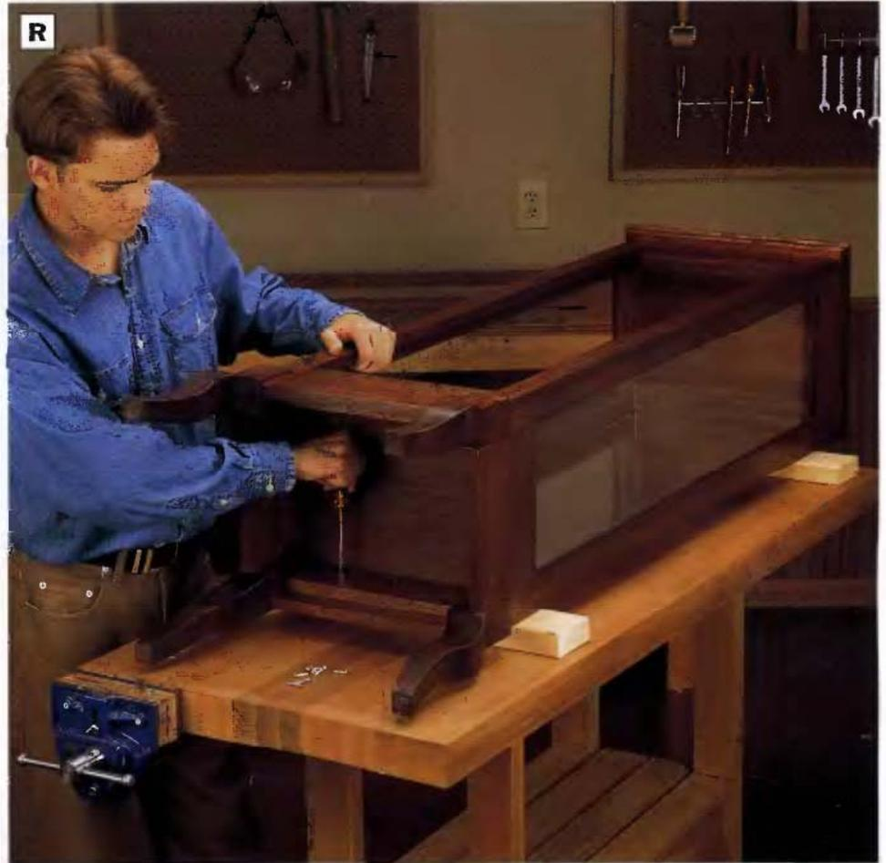
**PHOTO R:** Attach the base to the cabinet with screws driven through the pilot holes. Set blocks beneath the cabinet to allow clearance for the base.
