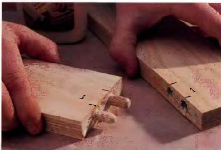
**3** After drilling all the holes, apply a dab of glue into each hole. Also apply glue to the mating wood surfaces. Slide the dowels into the holes to make the joint.
