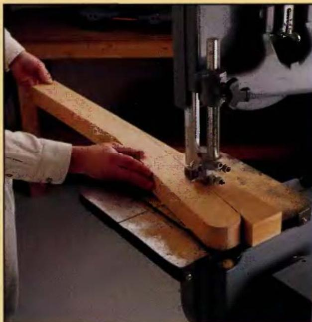
**RIP-CUTTING WITH A BAND SAW:** Like jig saws, a band saw can make "rip" cuts that generally follow the grain of the wood but aren't necessarily straight or parallel to the edge of the board. You can also make "true" rip cuts that are parallel to the edge using the fence that comes with most bandsaws. The edges of the cut won't be as sharp as a table saw cut, however.
