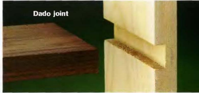
**DADO & RABBET JOINTS** interlock to add strength and increase glue surface. There are many variations of the joint, including the dado joint, (above) the rabbet joint (page 65, top left) and the combination dado/rabbet joint (page 65, top right).
