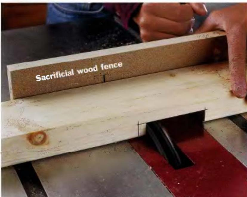
**USE A DADO BLADE.** A dado blade set installed in your table saw is the fastest tool for cutting notches in stock to create lap joints. Set the dado blade to its maximum cutting width and set the cutting height to equal the depth of the notch. Attach a sacrificial wood fence to the miter gauge for your table saw. Hold or clamp the workpiece securely against the fence so the area to be notched is clear of the miter gauge. Cut through the stock and the fence in several passes.
