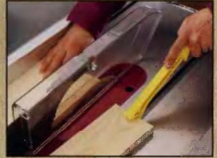
**3** When the blade cuts the board in two, push the workpiece past the blade with your right hand until it clears the blade on the outfeed side. Slide the cutoff piece away from the blade with your left hand or a pushstick to prevent it from coming in contact with the blade.
