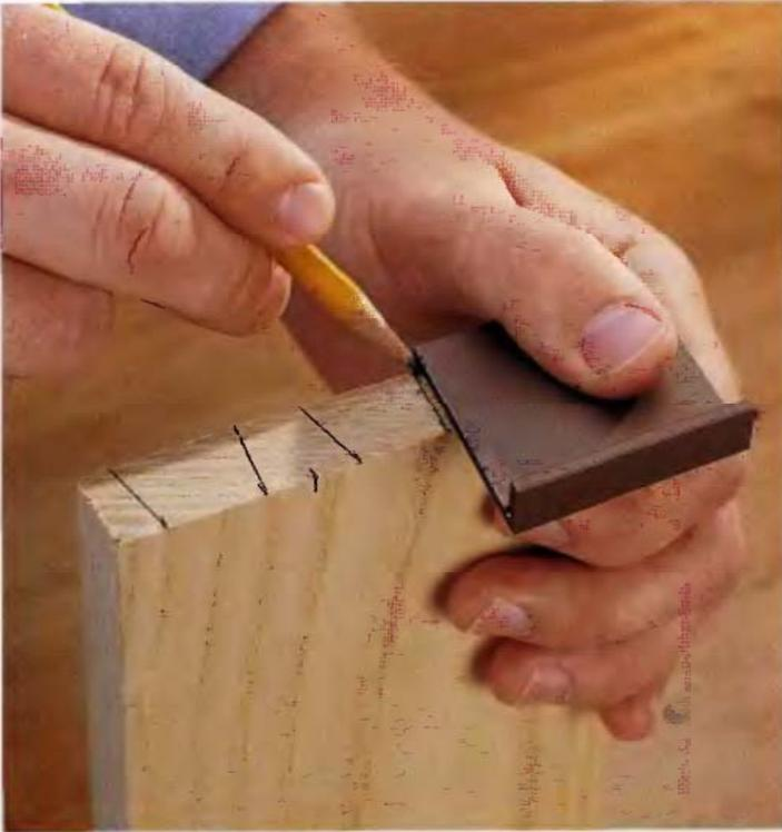
**OPTION:** Use a flanged dovetail layout jig to mark the dovetail pins. These inexpensive little devices can be found in most woodworking stores and catalogs. They're easy to use and yield consistent results. The only real drawback to these jigs is that they're not adjustable, and dovetails aren't a one-size-fits-all joint.
