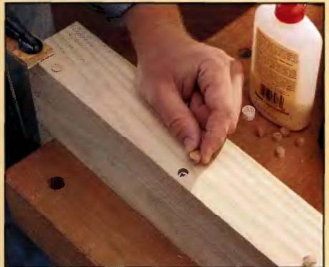
**2** Drive the screw, then apply glue to the end of a wood plug and insert it into the counterbore hole.
