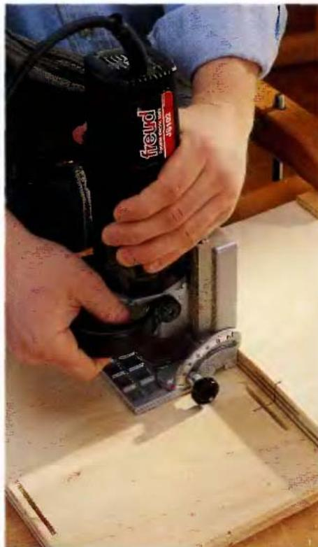
**2** With the workpieces still clamped together, cut matching slots in the other workpiece, using the reference lines to align the biscuit joiner.
