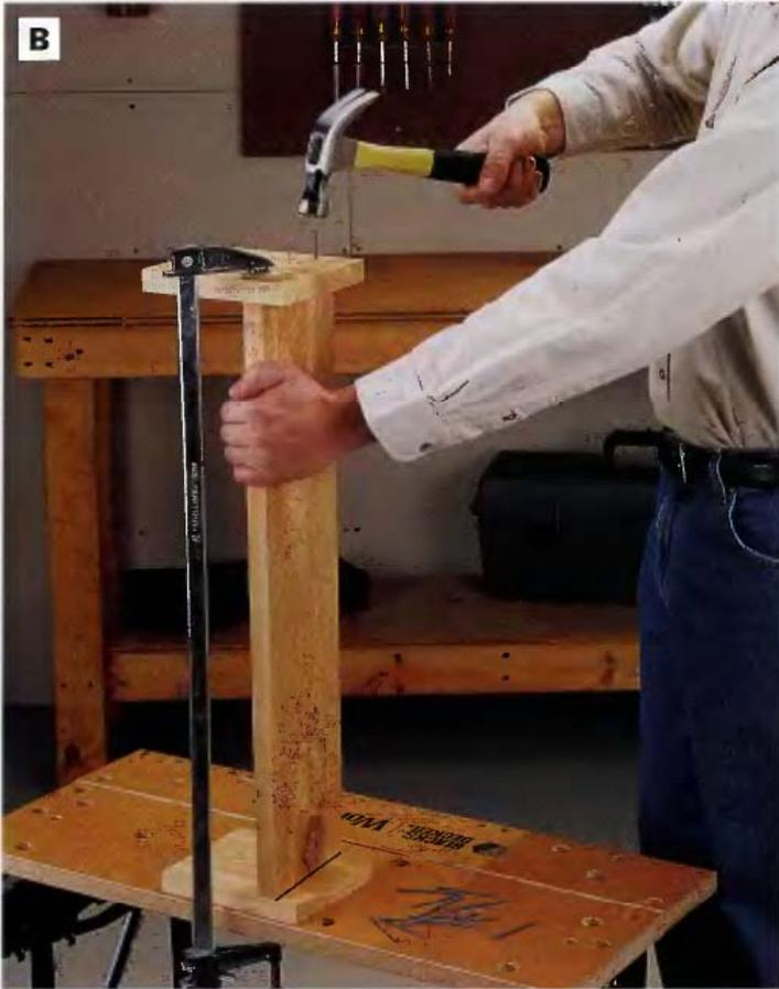
**PHOTO B:** Mark the slope of the bottom piece on the planter end pieces, then attach the ends to the bottom with galvanized finish nails. Clamp the pieces to help hold them steady during assembly.
