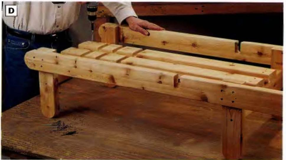
**PHOTO D:** Fasten the back supports to the seat stretchers. Leave 4½-in. spaces between the back supports and the legs to provide clearance for the chair back rails and adjustment braces.
