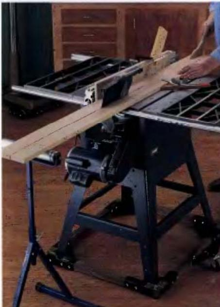
A **TABLE SAW** is the most heavily used tool in most woodshops. It can make just about any straight cut, including bevels and miters.
