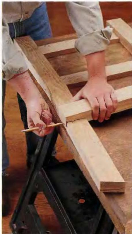
**CHAIRS AND BENCHES.** Lap joints are very often used to join the arms and/or spreaders of a chair base to the legs. The fitted nature of the joint provides good resistance to downward stress.
