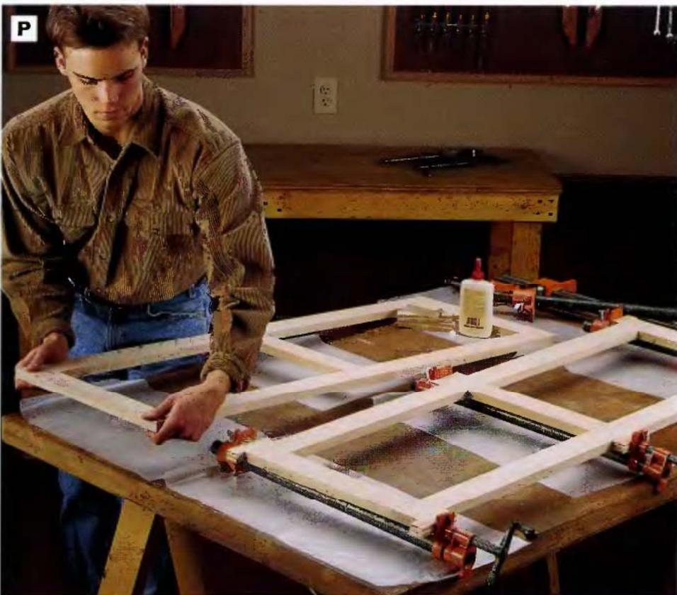
**PHOTO P:** Make dowel joints at all the rail/stile joints on each cabinet door, then glue the joints and assemble the door frames. Position a bar or pipe clamp beneath each rail location and use clamp pads to protect the wood.
