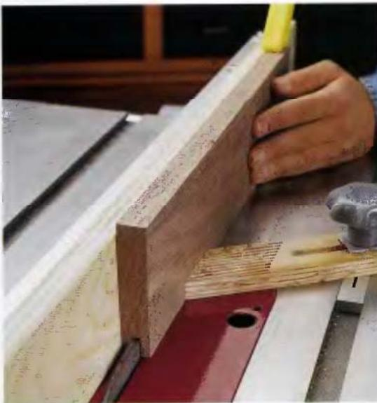
**3** Flip the workpiece and remove the waste on the other side of the tongue.
