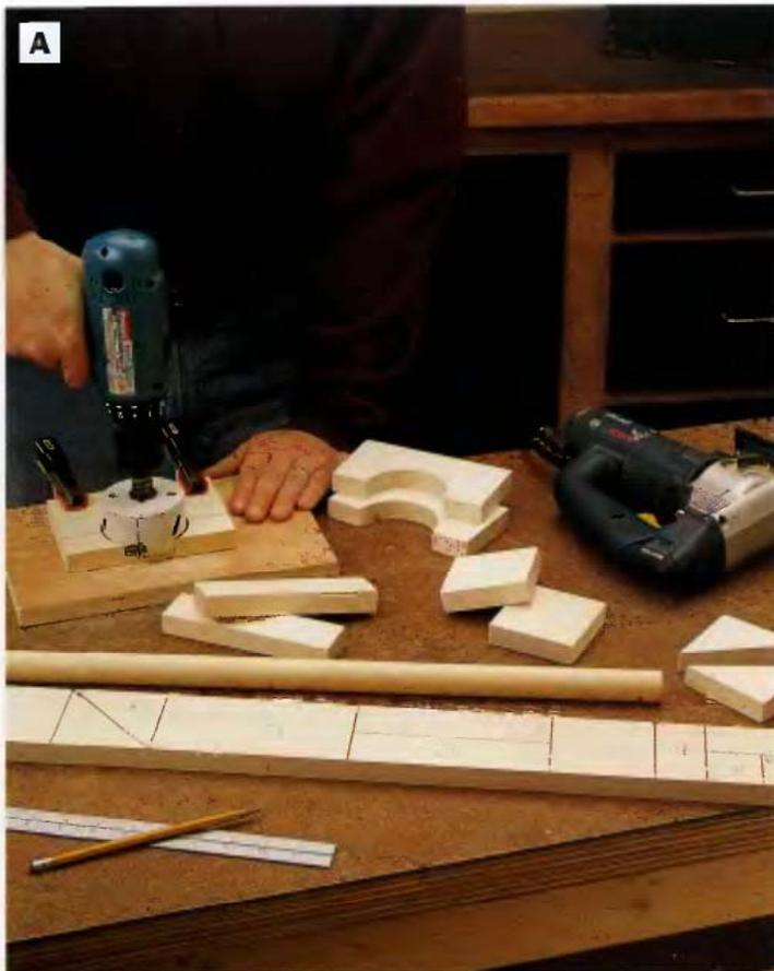
**PHOTO A:** Lay out and cut the block shapes. Arrange the parts on your boards to maximize the lumber. We cut the curved profiles of the arch blocks with a 3-in. hole saw.
