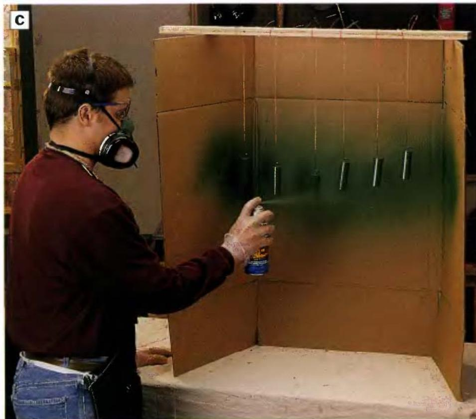
**PHOTO C:** Finish the blocks. We used primer and child-safe enamel spray paint. To make spraying easier, we hung the blocks with thumbtacks and string attached to a scrap of wood and suspended over a cardboard spraying shield. Wear a respirator if you use a spray finish.
